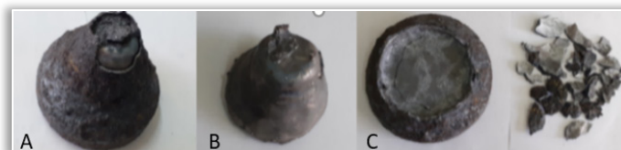
Figure 6. A) Products obtained, B) Metal, C) Slag
