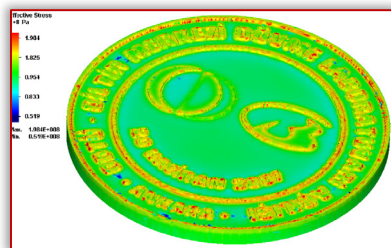
Figure 14. Effective Stress Distribution in the coin with a Diameter of 89mm
