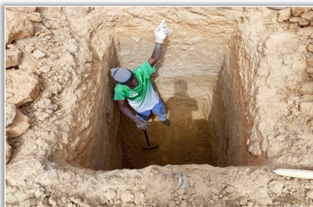
Figure 2. A typical excavated trial pit for soil sampling and in situ field observation.
