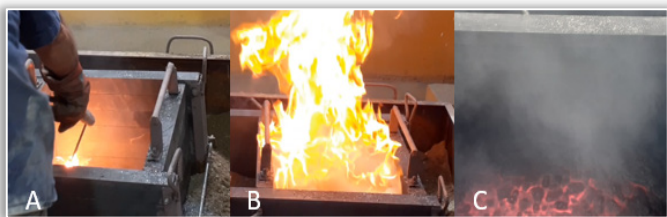
Figure 4. Obtaining of the thermites at the experimental pilot plant level: A) Ignition of the reaction, B) Self-sustainability of the reaction, C) Cooling of the thermite
