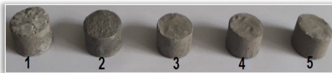
Figure 8. Test tubes manufactured with the 5 particle size fractions obtained
