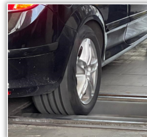
Figure 4. Dynamometer rollers in motion, testing the braking efficiency
