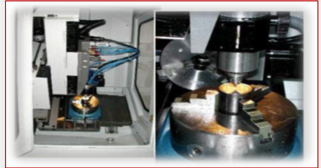
Figure 6. A view of mechanical engraving using a CNC machine
