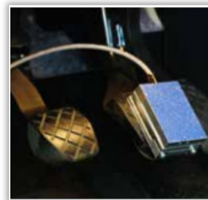
Figure 5. Brake pedal force measurement sensor [12]
