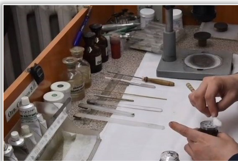
Figure 8. Manual polishing of coin dies
