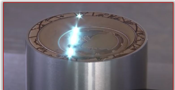
Figure 7. A view of laser engraving using a CNC machine
