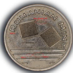
Figure 23. security features using laser micro-engraving
