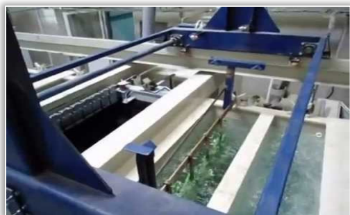
Figure 10. A view of the chrome plating process of the dies
