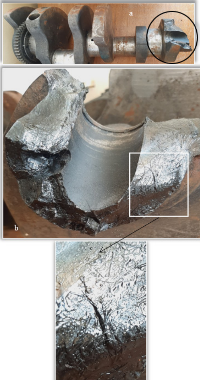
Figure 3. Destroyed cast iron crankshaft from a truck: a) general appearance and place of destruction b) secondary crack "closed type"
