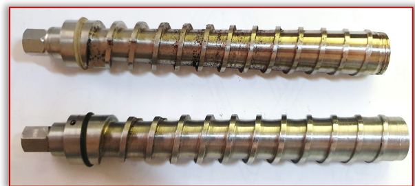
Figure 4 – Two screws with different pitches
