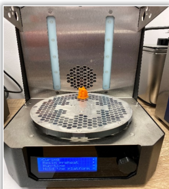
Figure 13. The part at the end of the curing process
