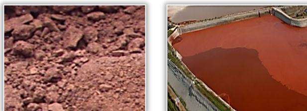
(a) (b) Figure 4. Red sludge generated in the alumina manufacturing process [2] a – red sludge; b – red sludge tailings pond
