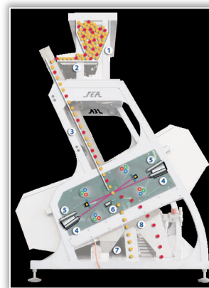
Figure 1 – The principle of operation of the optical seed sorting equipment, SEA (www.geangu.ro; www.cimbria.ro)
