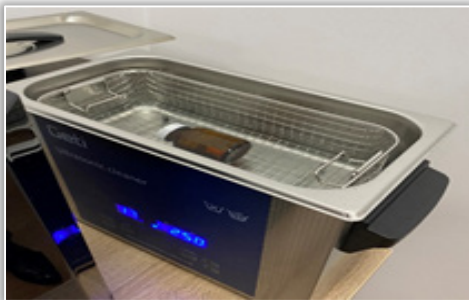
Figure 12. Cleaning of the part in ultrasonic bath with IPA
