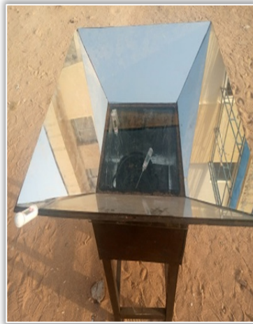
Figure 4: Developed box–type solar cooker: (a) Complete view, (b) Top view
