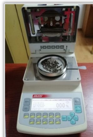
Figure 2 – Determination of moisture content with thermobalance AXIS –100
