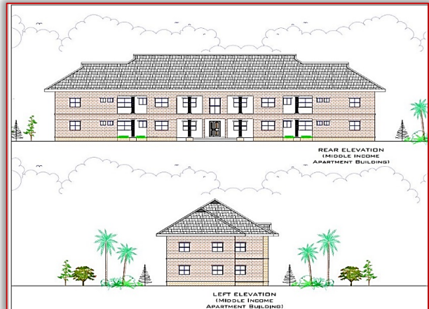
Figure 16: Rear and left elevations of middle income earners' apartment building
