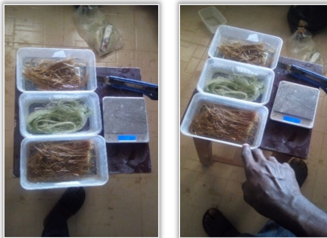
Figure 2. Alkaline treatment of the fibres NaOH
