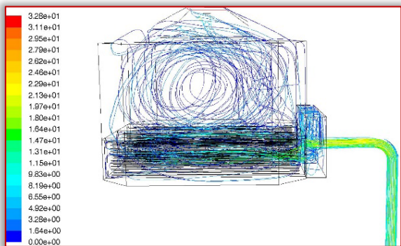
Figure 6 – The velocity pathlines of the warm air inside the drying equipment without hemp seeds
