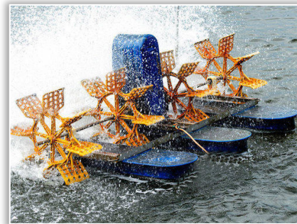
Figure 3 – Designs of paddle wheel aerator (Subha M. Roy 2021; https://www.indiamart.com/proddetail/aquaculture-paddle-wheel-aerator-20206411230.html )
