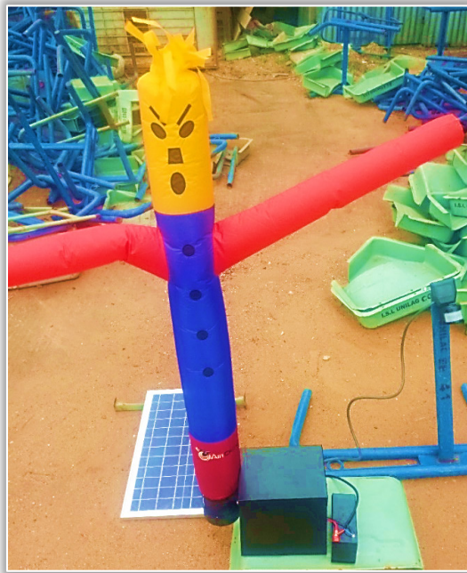
Figure 7: The set-up of the renewable energy avian pests' scarer
