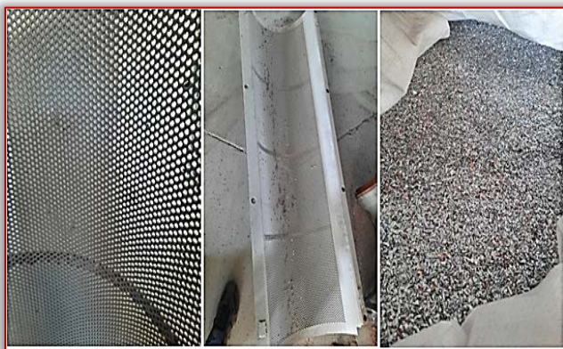
Figure 4. Al (Ø8) cable processing sieve and aluminum granules
