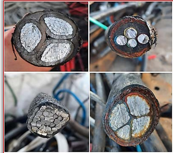
Figure 2. Different types of aluminum cables
