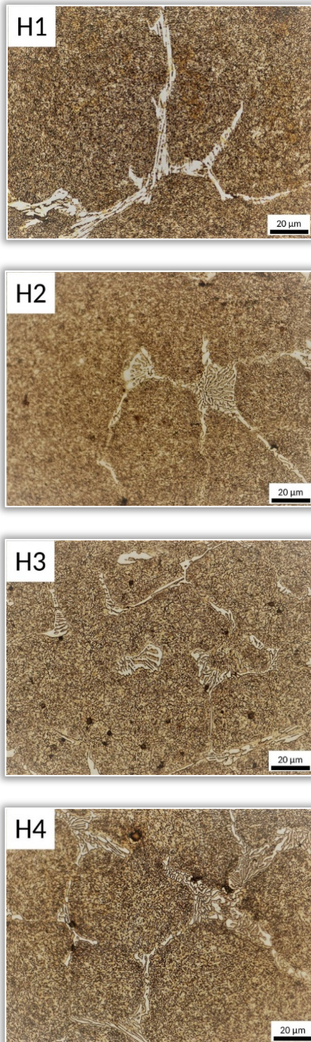
Figure 2. Optical Micrographs of Double Austenitization H1–H3
