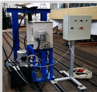
Figure 2 – Experimental model of lignocellulosic waste tableting equipment
