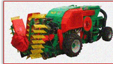
Figure 7. FUTURA 100 Self-Propelled Combine, a) in working position, b) in moving position ( https://utilajenucifere.wixsite.com )
