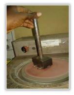
Figure 6: Test specimen under wear test
