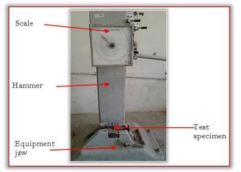
Figure 2: Izod impact test on test specimen
