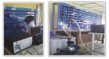
Figure 2: Fluid Friction Factor Board Set Up for Venturi Tube Meter
