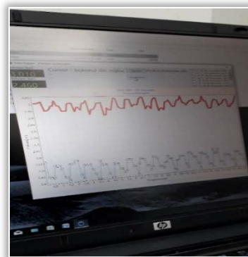
Figure 5. Acquisition of data regarding the variation of pressures in the connection points of the device to the main pipe of the stand (the equivalent of the main pipe of the localized irrigation system)
