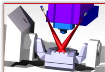
Figure 1. Mesasuring devices for on-machine measurement
