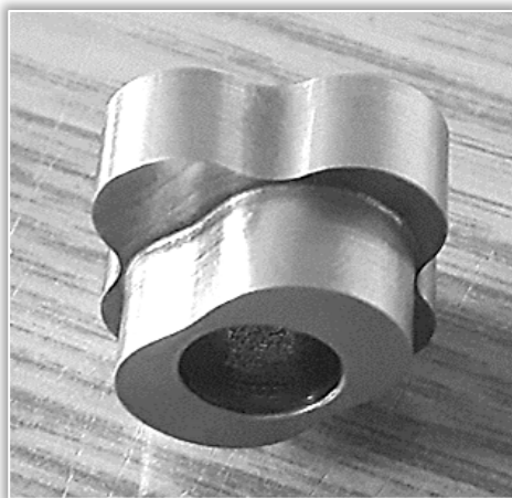
Figure 1. Small cycloid stepped planets
