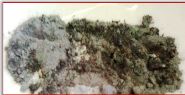
Figure 3. Mixture material (anode and cathode powder)
