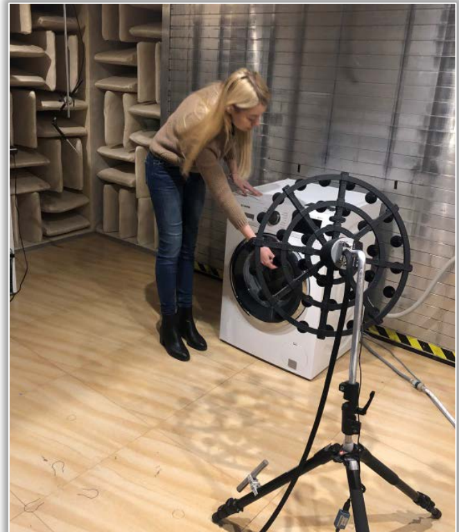
Figure 2. A view of the measurement with an acoustic camera in an anechoic chamber
