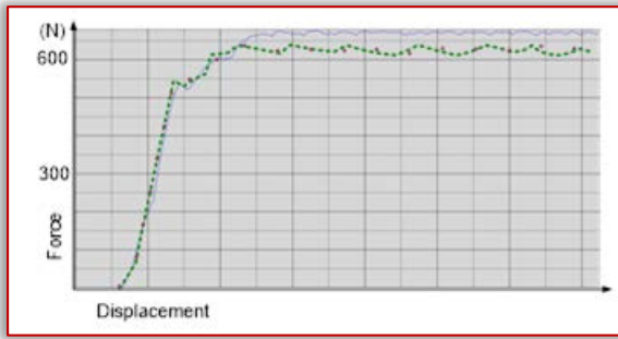
Figure 6. The reaction forces during the forming process (green dots: 3D shell, blue line: axisymmetric solid, purple dots: axisymmetric shell)
