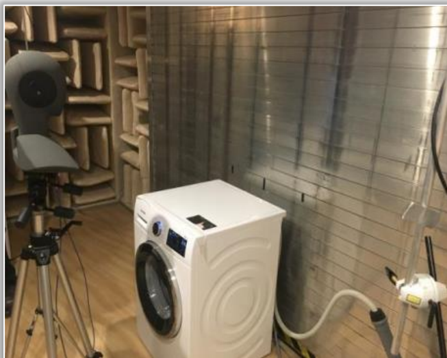
Figure 4. View of the measuring point in the anechoic chamber
