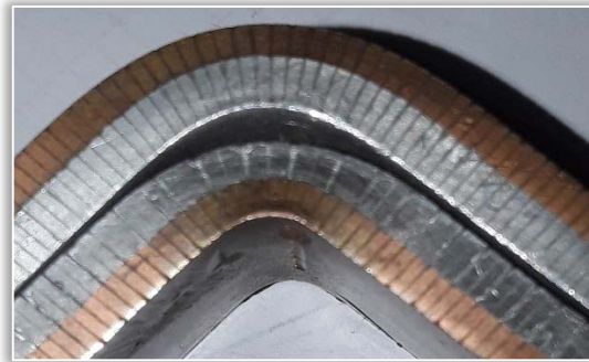
Figure 5. The layers of the laminar double–composites after bending force and their deformation after the experiment was performed in two bending cycles
