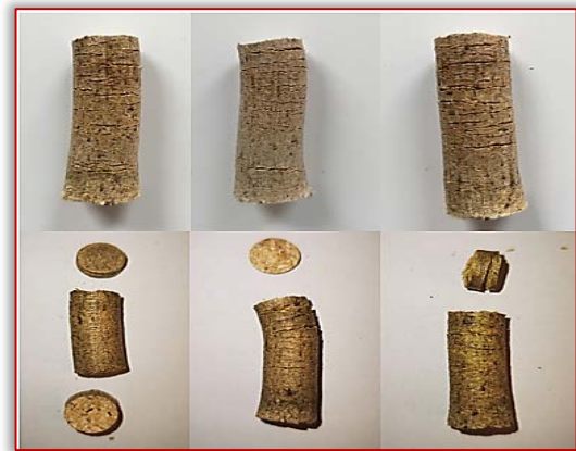
Figure 2 – Examples of broken pellets (in the first day – up, and in the day they broke – down)
