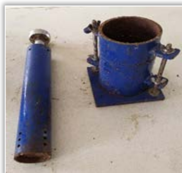
Figure 2. Determining the compaction
