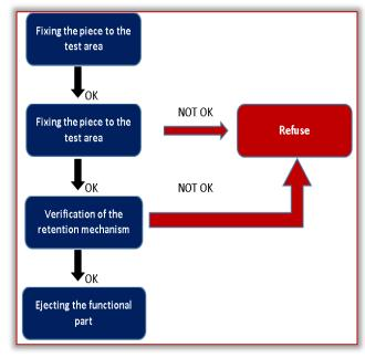
Figure 1. The operating algorithm of the mechatronic test system
