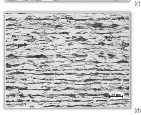
Figure 2: An example of structure in the middle of wall thickness: undeformed in the initial state a) and after deformation, b) in the orthogonal plane, c) in the tangential plane, d) in the parallel plane
