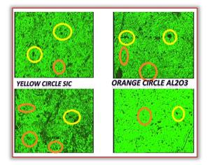
Figure 9: Vickers' Hardness test indentation photos
