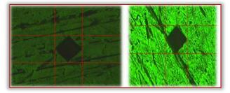
Figure 10: Vickers' Hardness test indentation photos [without heat treatment]
