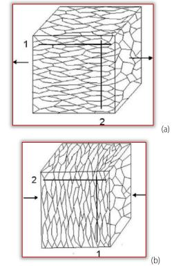
Figure 4: Anisotropic structure due to various types of deformation– linear a), planar b)
