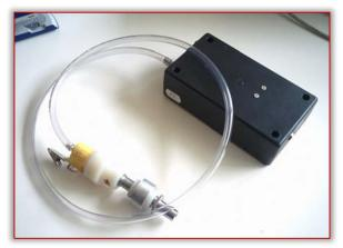
Figure 1: Personal sampling unit with pump
