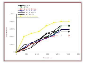
Figure 5: Water Absorption Curve for HDPE, EVA and HDPE/Silica Composites
