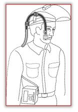
Figure 2: Placement of the sampling unit
