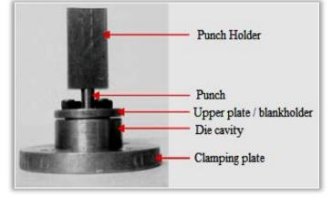
Figure 3. Micro deep drawing -Die assembly
