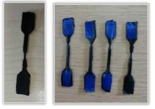
Figure 4. The first set of specimen before and after the tensile tests
