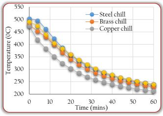
Figure 4: Cooling curves of aluminium alloy during solidification
