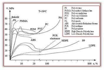
Figure 1. Tensile test diagrams of different polymers [Gunczer, 2009]
