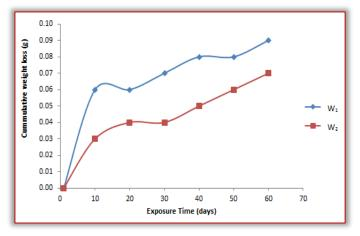
Figure 2: Variation of Cumulative Weight Loss with Exposure Time of Samples Immersed in Distilled Water
