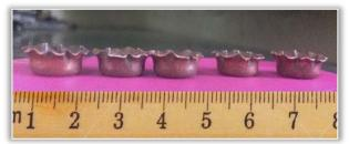
Figure 4. Cups formed with different initial thickness
