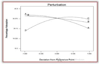
Figure 3: Perturbation plots for Cr(VI) adsorption onto ZnO
