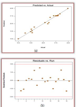
Figure 2: Plots of (a) the predicted against the actual experimental values and (b) the Studentized residuals against predicted values for Cr(VI) adsorption using ZnO
