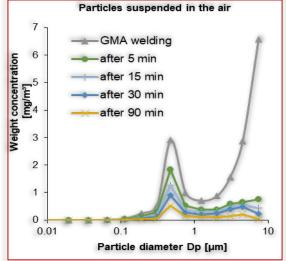
Figure 7: Result ELPI measurement - Particles in the air after finishing welding
