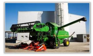
Figure 5 – Combine of harvesting hemp seeds, stems and leaves [2,3] HempFlax, a Dutch company established since 1994, is designing, developing and patententing equipment specialized in hemp cultivation, offering an innovating combine able to perform three different harvesting operations at the same time, namely hemp
