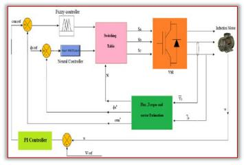
Figure 4. DTC with regulators hysteresis based on neural and fuzzy logic
