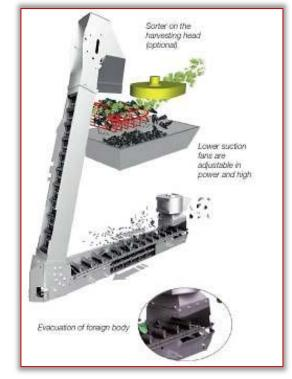
Figure 7 – Sorting and cleaning system (https://pellenc.com/) RESULTS
