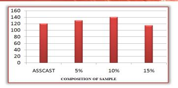
Figure 12: Graph plotted for Vicker's Hardness Number v/s Compositions of Specimens [with heat treatment]
