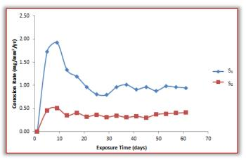
Figure 4: Variation of corrosion rate of samples S1 and S2 with the exposure time in days
