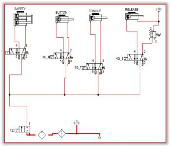
Figure 2. Pneumatic test bench system [4] Simulation of the pneumatic system of Figure 2 was made using a logic element and coils connected to each other at 24V and 0V and actuated by a button as shown in Figure 3.
