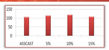
Figure 8: Graph plotted for Vicker's Hardness Number v/s Compositions of Specimens [without heat treatment]
