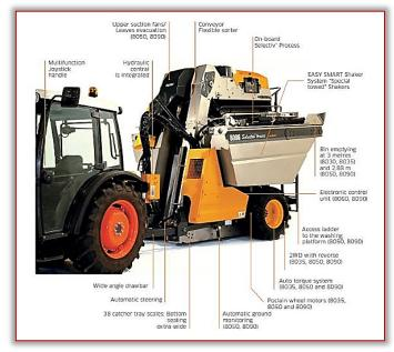
Figure2 – Towed harvester – PELLENC (https://pellenc.com/) Many winemakers prefer grapes, especially white varieties such as Sauvignon blanc, to be harvested by hand. Much progress has been made, however, in handling berries with a softer touch. An example of this is the used of extended beaters by means of which berries
