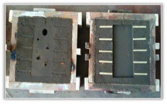
Figure 1: Sand mould with chills
