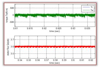
d) Strategy 3 with neural and fuzzy controllers of classical DTC Figure 18. Comparison between the classical and proposed strategy of DTC with neural and fuzzy controllers
