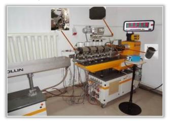
Figure 2 – Extrusion plant type "ZK 25", production Collin
