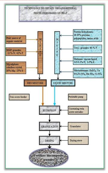
Figure 1 – Diagram of technological process for obtaining granular organo–mineral fertilizers based on peat.
