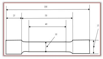
Figure 3: Dimension of the tensile test sample (mm)
