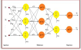
Figure 5. A Multilayer perceptron network with one hidden layer The inputs xk, k = 1...K to the neuron are multiplied by weights wki and summed up together with the constant bias term  $\theta$ i. The resulting in is the input to the activation function g. The activation function was originally chosen to be a relay function, but for mathematical convenience a hyperbolic tangent (tanh) or a sigmoid function are most commonly used. The mathematical model of a neuron is given by (17) [7]:
