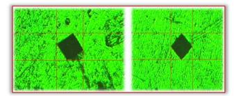
Figure 11: Vickers' Hardness test indentation photos [with heat treatment] Table 3: Vickers' hardness number for specimens
