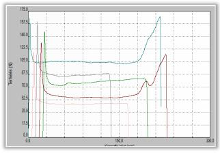
Figure 5. Tensile test result of PE-K001 (1-5) composites
