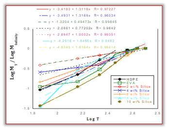
Figure 7: Diffusion Curve Fitting for Neat HDPE, EVA, and HDPE/Silica Composites
