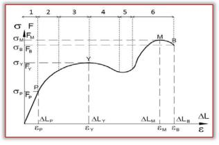
Figure 2. General plastic tensile strength diagram with six stages [Pék, 2000]
