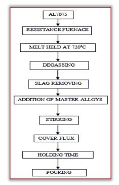
Figure 1: Activity chart of stir casting process Table 1: Density test calculation
