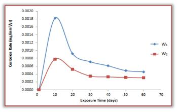
Figure 5: Variation of corrosion rate of samples W<sub>1</sub> and W<sub>2</sub> with the exposure time in days
