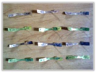
Figure 1. Micro tensile test – copper C1100 foil
