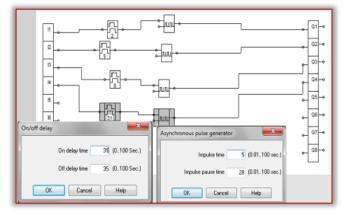
Figure 4. Impulse and time delay generators [4]
