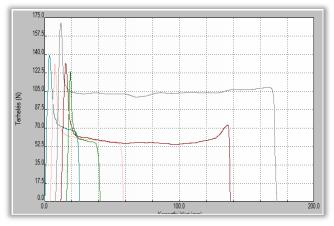
Figure 6. Tensile test result of PE-K002 (1-5) composites
