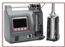
Figure 3: Dekati ELPI – cascade impactor
