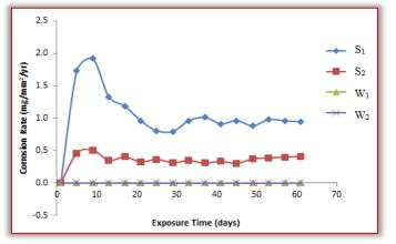
Figure 6: Variation of corrosion rate of all samples with the exposure time in days.
