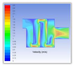
Figure 3: Velocity distribution in the 3D model
