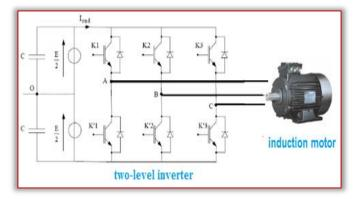
Figure 1. Voltage source inverter scheme
