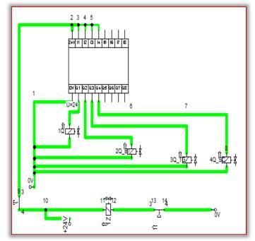
Figure 3. Electrical system of the test stands [4] For the electrical system to work inside the logic element we used 4 pulse generators and 4 time delayers as in Figure 4.
