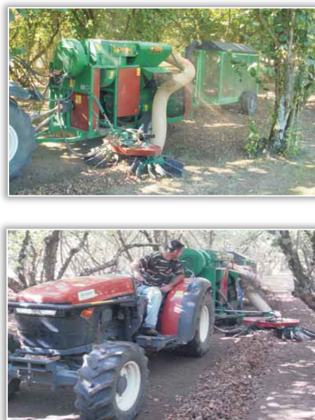
Figure 2 - General view of trailer type pneumatic nuts collection machines
