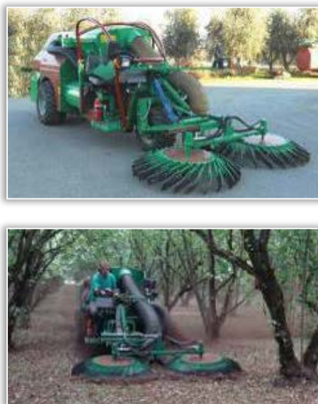
Figure 3 - General view of self-propelled type pneumatic nuts collection machines
