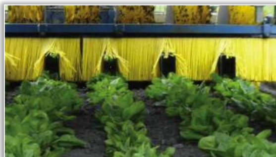
Figure 8 –Fobro Hoe Brush tunnel cultivator detail (AGB)
