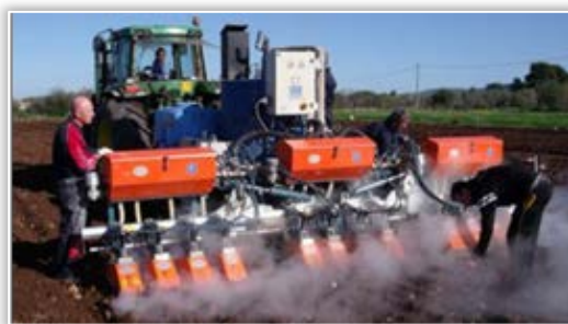
Figure 4 – Machine for soil disinfection in strips (prototype) (Raffaelli et al. 2016)
