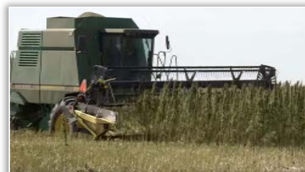
Figure 10 - Shortening the hemp with windrower [11]
