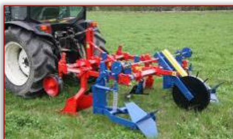
Figure 10 - Equipment for soil modelling in furrows compartmented on fruit and vineyard plantations, simultaneously in two furrows per interval. PCMV2.2 + EMBC2-0 [6]
