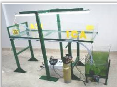
Figure 7 - Installation for open system growth of algae of waterfall type - ICA: 1. flat reactor; 2. collector; 3. illuminating system; 4. recirculation system; 5. CO 2 feeding and Ph control system; 6 agitators. a) appliance diagram; b) functional model ICA
