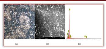
Plate 3: Micrographs of Al -6wt. % Cu 300 mm pouring height (a) optical (b) SEM and (c) EDS
