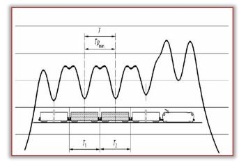
Figure 3. Time course of the equivalent sound level A The time interval for specific measurements was determined according to the length of the set (number of carriages). **RESULTS OF THE PASSING TRAIN MEASUREMENTS**
