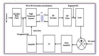
Figure 1. Circuit diagram of a closed loop model SMPS system DESIGN OF THE MODIFIED CONVERTER
