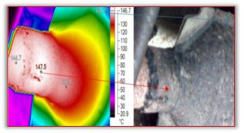
Figure 3. Infrared image of the exhaust system and real shot of the exhaust system
