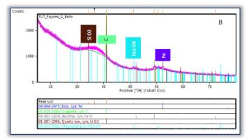
Figure 2. XRD image of coconut shells (Bello, et al., 2016) Table 1. Samples formulation
