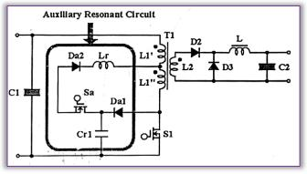
Figure 2. NPC-ARS auxiliary switch
