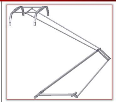
Figure 7. Maximum angular position for opening the pantograph mechanism (pantograph higher position)
