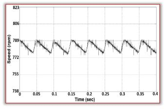
Figure 18. Experimental Result for Step Response of Speed of BLDC Motor for a reference speed of 785 rpm under 50% of Full Load
