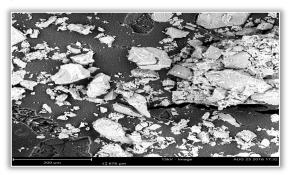
Figure 8a. SEM micrograph of 40 wt. % SP reinforced carbon composite
