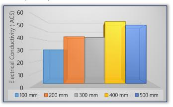
Figure 5: Electrical Conductivity of Al6wt%.Cu Alloy at Varied Pouring Height
