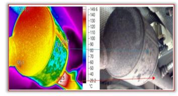
Figure 2. Infrared image of the exhaust system and real shot of the exhaust system
