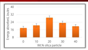
Figure 6. Variation of impact energy with silica particle additions
