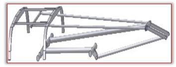
Figure 6. Minimum angular position for opening the pantograph mechanism (pantograph lowered position)
