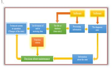
Figure 1. The process of maintenance management using information system for maintenance
