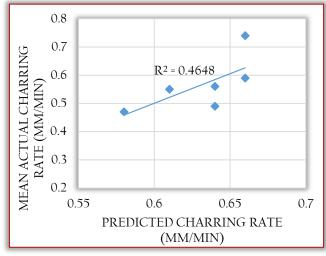
Figure 8: Linear correlation for samples exposed to 20°C to 300°C (9% MC, 0-60 minutes)
