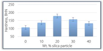
Figure 5. Variation of hardness with silica particle additions • Impact energy
