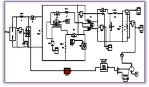
Figure 3.7. Modified converter using fuzzy logic
