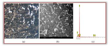
Plate 5: Micrographs of Al -6wt. % Cu 500 mm pouring height (a) optical (b) SEM and (c) EDS
