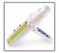
Figure 1: mini-Wright peak flow meter
