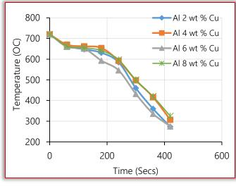
Figure 2: Cooling curves for Al-Cu alloy
