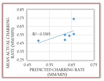
Figure 9: Linear correlation for samples exposed to 20°C to 300°C (12% MC, 0-60 minutes)
