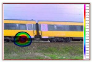
Figure 10. Acoustic image – 380 – 400 Hz
