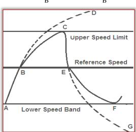
Figure 8. Transient speed response by the proposed controller The speed ripple thus can be found as:
