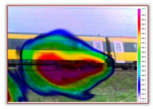
Figure 9. Acoustic image – chassis noise
