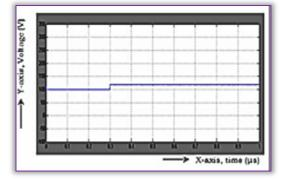
Figure 3.2. DC input voltage with disturbance Closed loop controlled modified forward converter is shown in Figure 3.4. DC input voltage with disturbance and DC output voltage with disturbance are shown in Figure 3.5 and Figure 3.6. Modified forward converter using fuzzy logic is shown in Figure 3.7. DC input voltage with disturbance and DC output voltage with reduced error are shown in Figure 3.8
