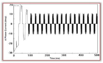
Figure 11. Simulated output of phase current waveform of the three phase BLDC motor employing the proposed on off controller on 30% of full load at 1153 rpm
