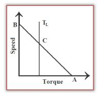
Figure 2. Speed-torque characteristic of BLDC motor
