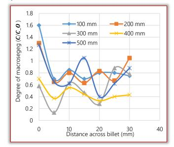
Figure 4: Effect of varied pouring height on relative segregation within AI - 6wt. % Cu Alloy
