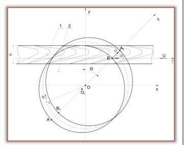
Figure 1: Scheme for determining the speed of movement of the circular saw in direction of the feed rate
