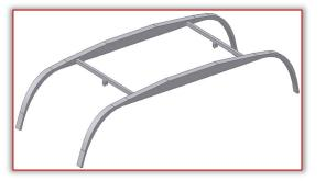
Figure 5. Pantograph sleigh
