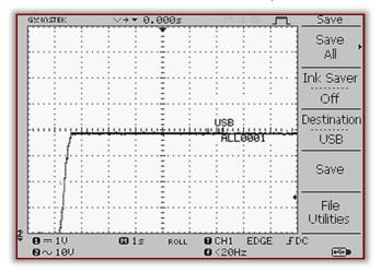
Figure 15. Oscillogram of experimental result for close loop step response of speed BLDC Motor on 30% full load and 1130 rpm
