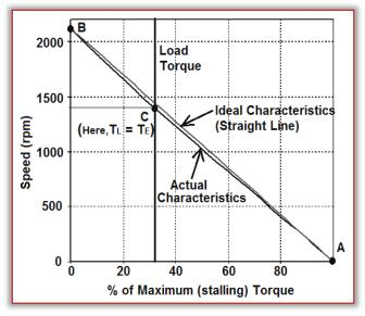
Figure 3. Simulated speed-torgue characteristics of BLDC motor
