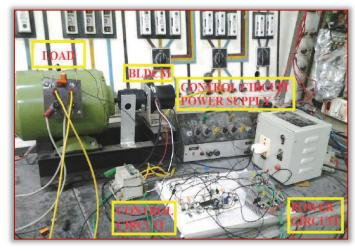
Figure 13. Experimental setup of BLDC motor drive scheme in laboratory
