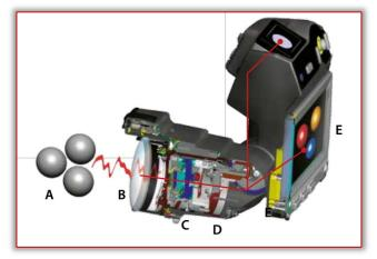
Figure 1. How thermographic camera works [4] Thermographic works as follows: Infrared energy (A) coming from the object is recorded using the detector (C) of the optics (B), the detector then sends the information to the | – Visual inspection of the exhaust system.
