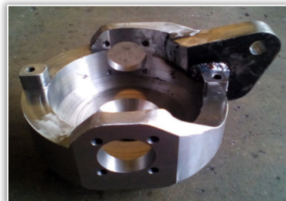
Figure 14. New mechanical part produced with milling and welding
