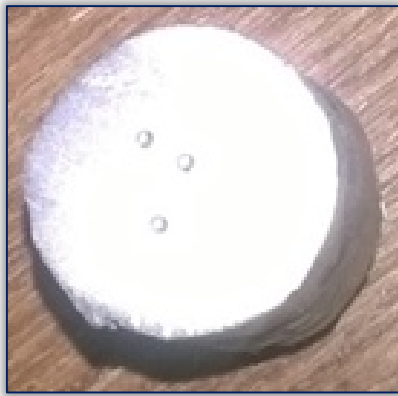
Figure 5. One of the Prepared Samples with Indentations
