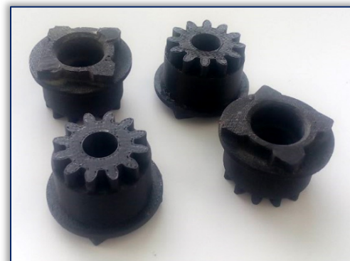
Figure 7. Small batches of gears made in the integrated process of additive manufacturing technology and vacuum casting
