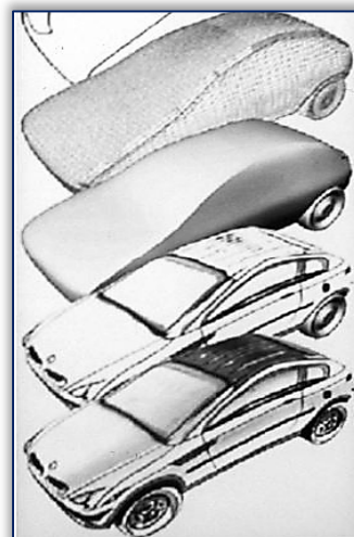
Figure 2. An overview of a vehicle design development, [3]
