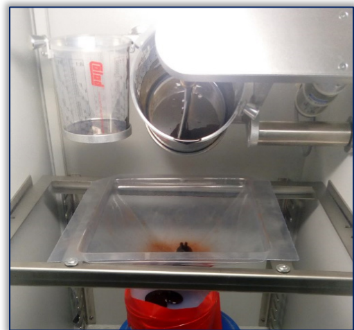
Figure 6. The casting process in a vacuum chamber MK-mini
