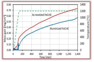
Figure 8. Relative mass gain as a function of oxidation time in air at 1200℃ (heating rate 20 K/min)
