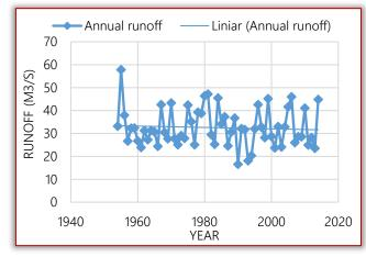
Figure 5. Linear runoff trend for Kratovska Stena station CONCLUSIONS
