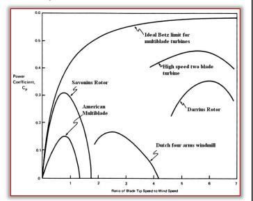
Figure 1. The power coefficient  $C_p$  as a function of the tip speed ratio for different wind machines designs. [7]
