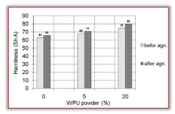
Figure 1. Results of hardness testing
