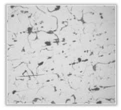
Figure 8: Microstructure of un-inoculated sample x50
