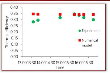
Figure 3. Thermal efficiency comparison between experimental and numerical results
