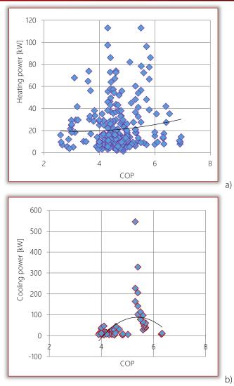
Figure 2. Dependence of the COP of the geothermal heat pump type earth - water on the heating and cooling power for all manufacturers (figures formed based on data from [10,11,12,13]). a) The COP dependence on the heating power for the collected data from 32 manufacturers of geothermal heat pumps; b) The COP dependence on the cooling power for the collected data from 32 manufacturers of geothermal heat pumps
