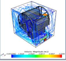
Figure 4. Representation of the fluid streaming in the drying chamber
