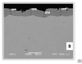
Figure 1. SEM image of FeCrAl (A) and NiCr alloy (B) aluminized at 670°C, 1.5 h
