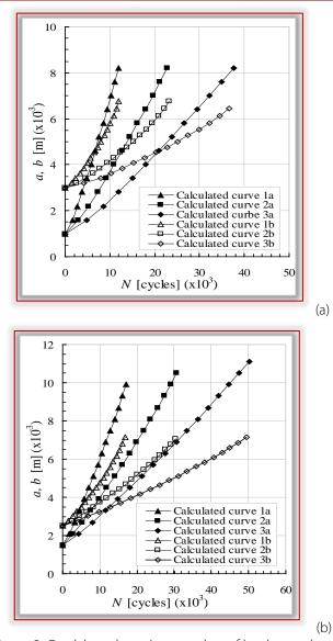
Figure 3. Crack length against number of loading cycles to failure: (a) the effect of thickness of the plate (w = 65 mm, 1 - t = 12 mm, 2 - t = 15 mm, 3 - t = 18 mm), (b) the effect of width (t = 10 mm, 1 - w = 50 mm, 2 - w = 65 mm, 3 - w = 80 mm). CONCLUSIONS
