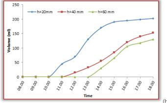
Figure 5. Comparison of (a) instantaneous volume of distilled water collected from the solar still with time (b) cumulative volume of distilled water collected from the solar still with time.
