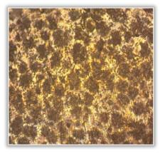
Figure 3: Eutectic cell 5.0 mm: x50
