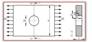
Figure 1. Geometry of the plate with quarter-elliptical corner crack emanating from a hole (a - depth direction, b – surface direction).
