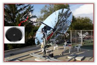
Figure 1. The examined solar dish collector
