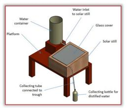
Figure 1. Experimental set-up of the solar water still. 🕒 Energy Received by the Solar Still
