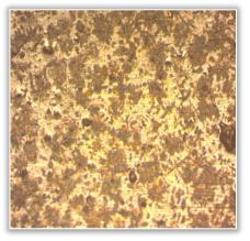
Figure 4: Eutectic cell 7.0 mm: x50
