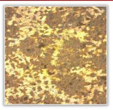
Figure 6: Eutectic cell 11.5 mm thickness x100
