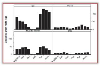
Figure 2. Monthly uptake of air pollutants by green roofs in Chicago between August 2006 and July 2007.
