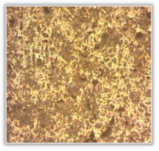
Figure 5: Eutectic cell 8.0mm thickness x100
