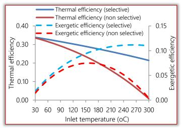
Figure 8. Thermal and exergetic efficiencies for the examined absorbers
