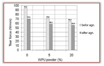
Figure 4. Results of tear resistance testing
