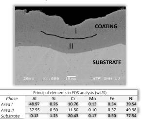
Figure 6. SEM-EDX analysis of NiCr coated at 730 °C for 1.5 h The coating on Fe-Cr-Al alloy is a dual phase mixture with dark and light areas. EDS analysis show that the dark phase is rich in aluminium and contain iron and a small amount of chromium. The light phase contains a smaller percentage of found out that Al<sub>3</sub>N<sub>2</sub> is the major phase because of a very high aluminium and iron, and a larger percentage of chromium. It diffusivity of Al<sub>3</sub>Ni<sub>2</sub>.
