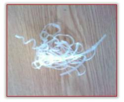
Figure 1. Measurement 1:  $(a_p=2 \text{ mm}; v_f=80 \text{ mm/min}; n=600 \text{ rpm})$
