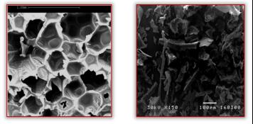
Figure 5. Appearance of PU before and after recycling
