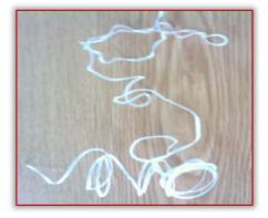
Figure 3. Measurement 3:  $(a_p=2 \text{ mm}; v_f=300 \text{ mm/min}; n=600 \text{ rpm})$
