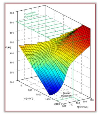
Figure 3 – Optimal cutting conditions searching procedure TBLO algorithm is initiated with randomly generated answers in predefined population of students. The student's answers are optimum solution candidates. ANFIS model predicts cutting forces for each of the student. Predicted maximal forces are used as an objective function which TBLO tries to maximize.
