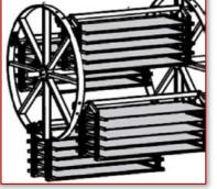
Figure 1. Representation of the rotary dryer interior
