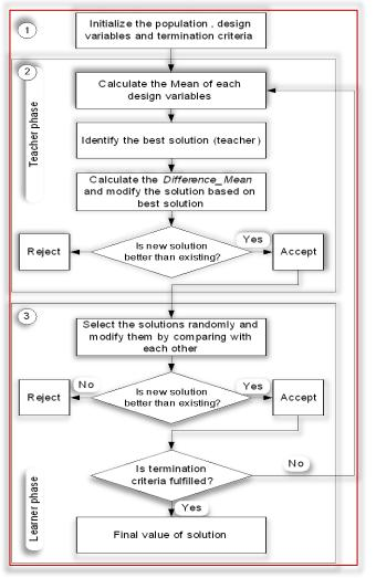
Figure 1 – The diagram of the TBLO algorithm
