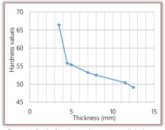
Figure 16: Graph of hardness values against wall-thickness
