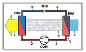
Figure 1. Principle of operation in a simplified heat pump dryer After flowing through the evaporator and condenser of the heat pump the dry and warm air is ready to flow into the drying chamber in which the material, which is to be processed, is being placed. The simplified heat pump dryer has two separated loops with common heat exchangers. The drying air loop (abcd) contains the air cooler (EVA), heater
