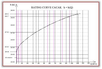
Figure 1. Rating curve for the station in Čačak
