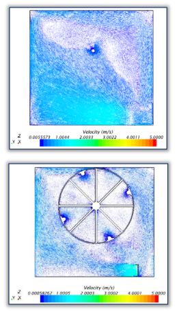
Figure 6. Left: Vector field of the speed alongside side wall, Right: Wheel.
