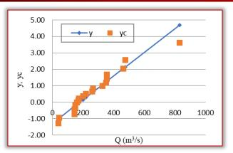
Figure 3. EV1 Gumbel for Čačak station Table 2. The maximum flow Qc values for Čačak for fixed return periods
