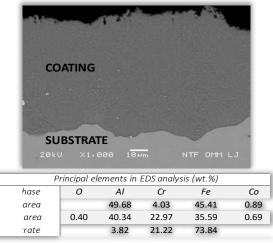
Figure 5. SEM-EDX analysis of Fe-Cr-Al coated at 730 °C for 1.5 h
