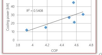
Figure 1. The dependence of the COP of the geothermal heat pump type earth – water on the heat (left) and cooling power (right) (figures formed based on data from [10,11,12,13]).
