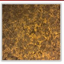
Figure 2: Eutectic cell 4.5 mm: x50
