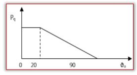
Figure 1. Diagram of thermal capacity decreasing with increasing ambient temperature
