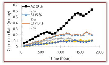
Figure 5: Variation of Corrosion Rate with Exposure Time for Mild Steel Coated in Red with 0-25% Zn Powder Addition
