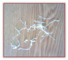
Figure 2. Measurement 2: (ap=2 mm; vf=80 mm/min; n=1200 rpm)
