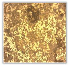
Figure 1: Eutectic cell 3.5 mm: x100
