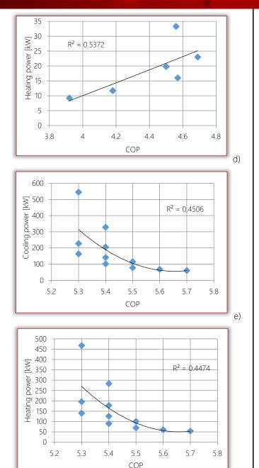
Figure 1 (continuing). The dependence of the COP of the geothermal heat pump type earth – water on the heat (left) and cooling power (right) (figures formed based on data from [10,11,12,13]). d) Bosch Logatherm WPS heat pump - the COP dependence on the heating power; e) Hidros heat pump - the COP dependence on the cooling power; f) Hidros heat pump - the COP dependence on the heating power
