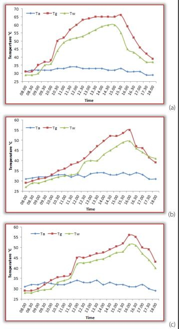
Figure 3. Variation of average temperature with time in the solar still for different days. a) Day 1; b) Day 2; c) Day 3
