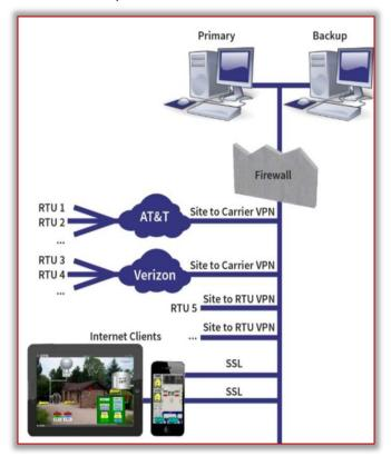
Figure 3. The hardware connection with back-up data
