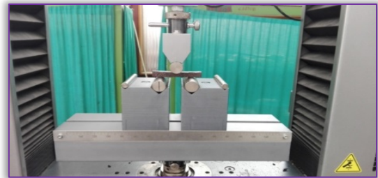
Figure 5. Sample mounted in the equipment to perform the bending test
