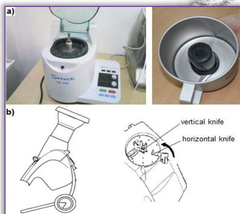
Figure 1 - a) Laboratory mill Grindomix GM-200 and b) Grinder for vegetable residues Viking GE150
