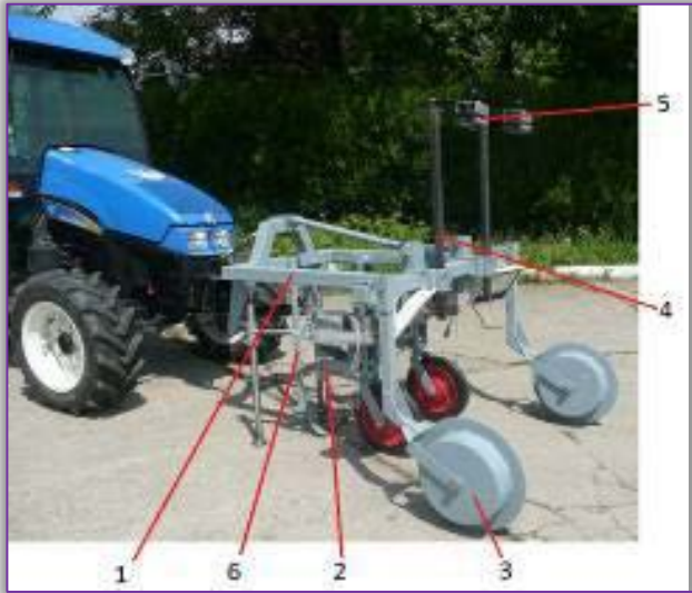
Figure 2. Experimental model IHE (1-frame, 2 - hoeing section, 3 - wheels of displacement and working depth adjusting, 4 - cameras supports, 5 - cameras, 6 - parking foot)
