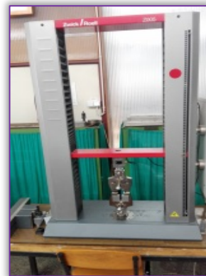
Figure 2. Assembly of Zwick / Roell Z005 equipment prepared for mechanical tests
