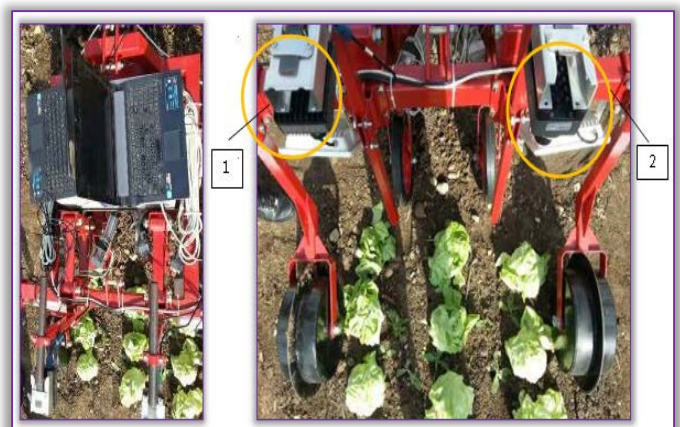
Figure 1. Image from experiment filed with IHE 1) black-and-white camera 2) colour camera
