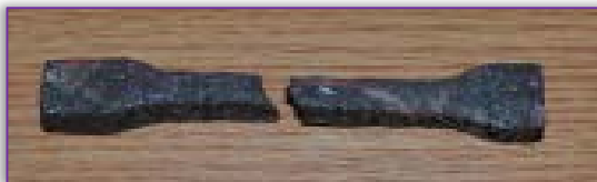
Figure 4. Sample broken after tensile test Table 2. Values of the samples parameters subjected to the tensile test
