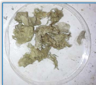
Figure 13: Fibers extracted at 100 ° C for 0.3mol/L of sodium hydroxide.
