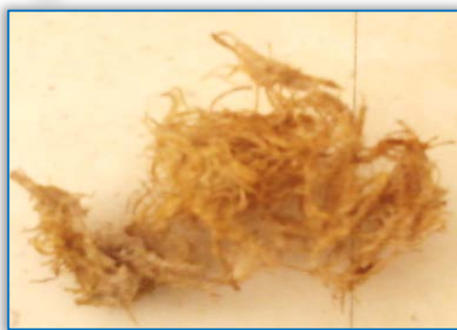
Figure 10: Fibers extracted at 60°C for 0.1mol/L of sodium hydroxide.
