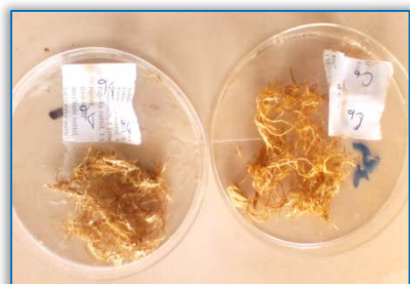
Figure 12: Fibers extracted at 80 ° C for 0.2mol/L of sodium hydroxide.
