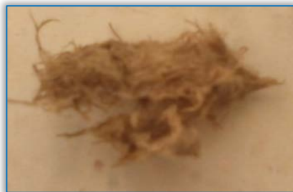
Figure 11: Fibers extracted at 60°C for 0.2mol/L of sodium hydroxide
