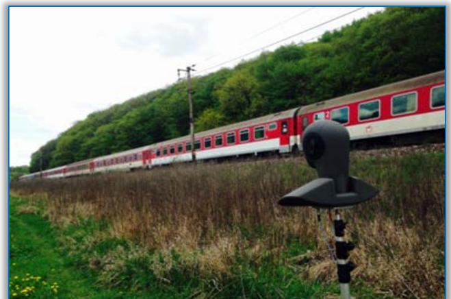
Figure 4. Psychoacoustic head turned toward the passing train
