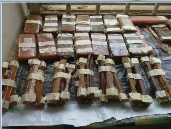
Figure 3: Composite samples after curing The following symbols were used to represent the various samples from the corncobs: Y-NaOH – Yellow corncob treated with NaOH; W-NaOH – White corncob treated with NaOH; Y-KOH – Yellow corncob treated with KOH; W-KOH – White corncob treated with KOH; U-Yellow – Untreated Yellow corncob; U-White – Untreated White corncob
