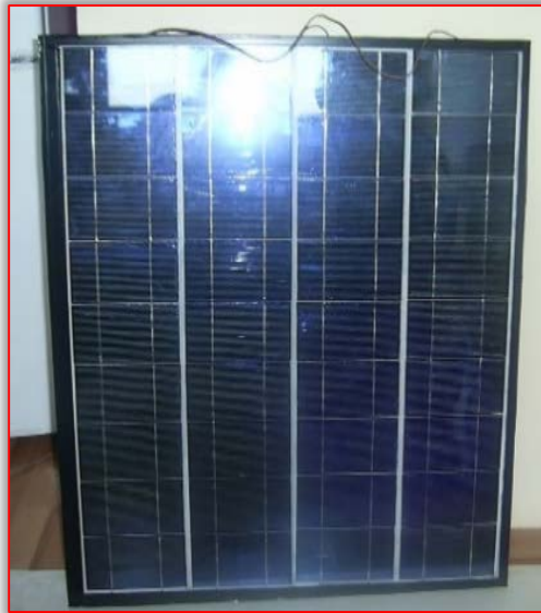
Figure 3. The first module – the photovoltaic panel [4-6] The first solar module consists of a handmade photovoltaic panel made from 36 solar cells that produces 65W and 3.6 A. [4-6]
