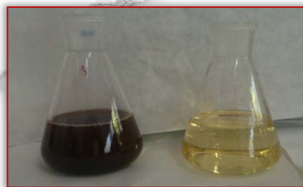
Figure 3. Sample of WW from the steam chamber before the treatment and after the second step of the treatment by ferrate (VI)
