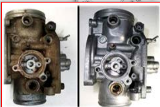
Figure 2. Example of US cleaning of product before and after cleaning
