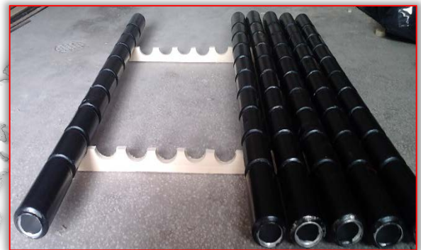
Figure 4. The second module – the panel from recycled aluminum soda cans [4,5]
