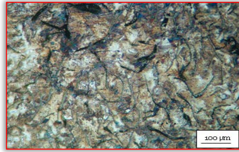
Figure 2. Microstructure of the base material of the cylinder head
