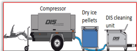
Figure 5. Equipment of dry ice cleaning [4]
