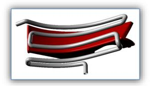
Figure 7. Several designs of the conformal cooling channels
