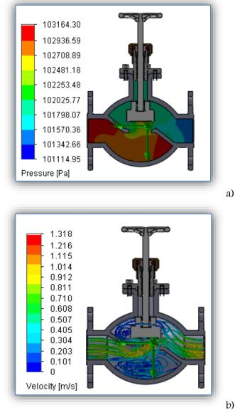
Figure 4. Variation of pressure (a) and velocity profile (b) for the case 3 of simulation;
