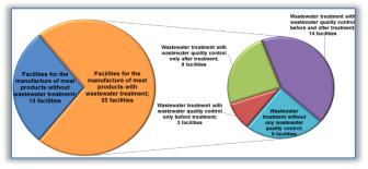
**Figure 5**. Wastewater treatment quality control in facilities for the manufacture of meat products
