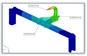
Figure 8-2: Area with maximum strain
