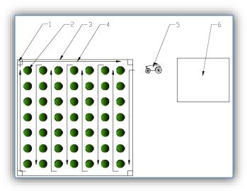
Figure 5. Description of the technological process. 1. Reference points Storage area - power supply; 2. Olive trees Robot; 3. Olive trees plantation; 4. Harvesting flow Reference point; 5. Robot – harvest machine; 6. Storage area, power supply and robot control room.
