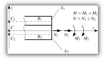
Figure 2. Normal forces and bending moments
