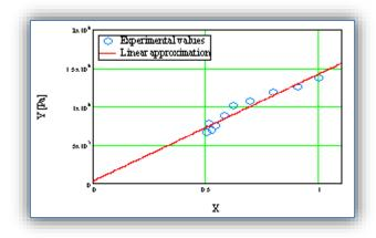
Figure 2: Y – X characteristic for rubber, obtained under uniaxial traction.
