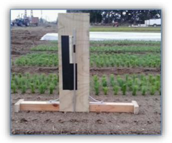
Figure 6 – Measuring device for hole depth and angle
