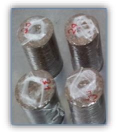
Figure 1 ~ Briquettes from oat biomass
