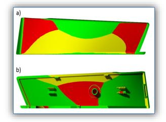
Figure 14. The comparison of the non-deformed (green), conventional cooled (red) and conformal cooled (yellow) cover
