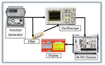
Figure 6. Hardware set-up for automation measurement
