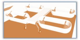
Figure 4: Drone body frame
