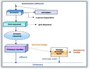
Figure 1. Diagram of a mechanical wastewater treatment plant
