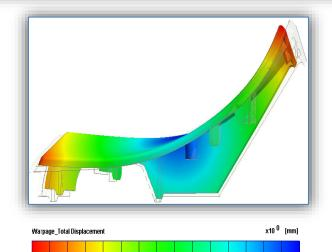
2.91 2.72 2.53 2.34 2.16 1.97 1.78 1.59 1.41 1.22 1.03 0.84 0.66 0.47 0.28 0.10 Figure 13. Warp behaviour of conventional cooled cover in scale 2
