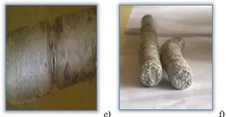
Figure 4: Representative photomicrographs showing the nature of macroscopic crack evolution to final fracture in the test specimen (a) after 4 days of testing, (b) for 9 days of testing, (c) 15 days of testing, (d) 25 days of testing, (e) 35 days of testing, (f) fracture on 40<sup>th</sup> day of testing
