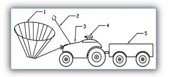
Figure 4. The concept of harvesting robot. 1. Net "umbrella"; 2. Shaker for olive tree; 3. Autonomous (or with driver) mobile platform; 4. Data transmitter and receiver with video camera; 5. Trailer for olives.
