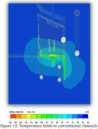
Figure 12. Temperature fields in conventional channels cooled mould after 20 sec. of cooling time (longitudinal cross-section)
