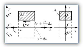
**Figure 3.** Equilibrium condition in z direction for a small beam element  $\Delta B_1$
