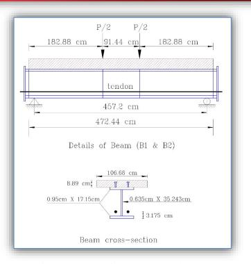
Figure 7. Composite beam (B1 and B2) The parameters and material properties of the simple prestressed composite beam are shown in Tables 1 and 2.
