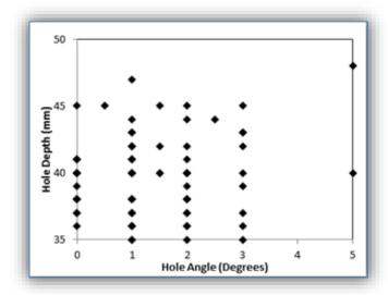
Figure 7 – Hole depth v hole angle for mechatronically dibbled Radiata pine seedlings
