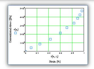
Figure 1: Stress – strain characteristic for rubber, experimentally obtained under uniaxial traction, [4, 5].
