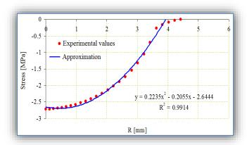
Figure 9:  $\sigma_v$  stress distribution corresponding to an imposed normal approach of 1.628 mm, for the contact model between a D = 12,6 mm - rubber ball and a rigid half-space.
