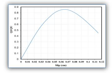
Figure 4. Load-slip curve from push-out test used in ANSYS model
