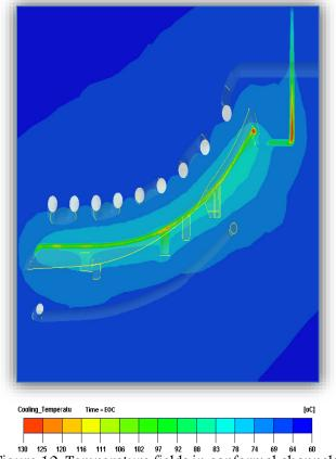
Figure 10. Temperature fields in conformal channels cooled mould after 20 sec. of cooling time (perpendicular cross-section)
