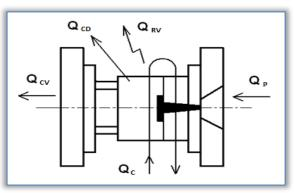
Figure 1. Thermal balance of injection mould
