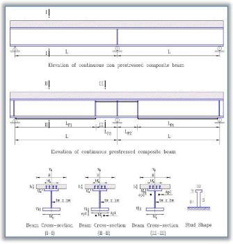
Figure 16. Continuous (two span) Composite beam without and with prestressing subjected to uniform load The mechanical properties, and section for concrete slab, and steel beam are summarized in tables 3 to 4. Also the distances from bottom and top steel flange and force in cable is show in table 5.
