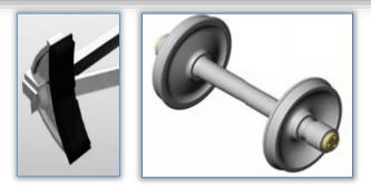
Figure 2. The friction pair (brake shoe – wheel)
