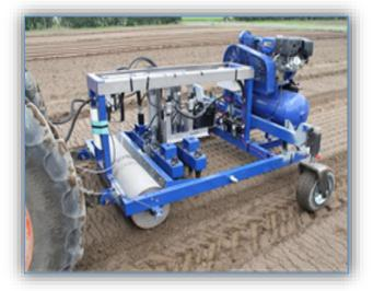
Figure 5 – Completed mechatronic dibbling machine during testing
