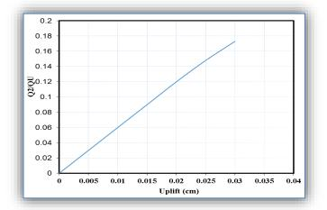
Figure 5. Load-uplift curve from pull-out test used in ANSYS model The equation for push-out curve [13] is:
