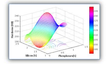
Figure 17. The regression surface, case of HB=f(Si,P)
