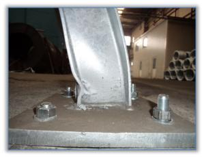
Figure 9: Pillar deformed on the edge
