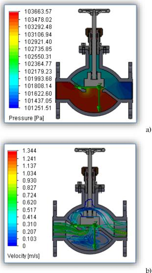
Figure 2. Variation of pressure (a) and velocity profile (b) for the case 1 of simulation;
