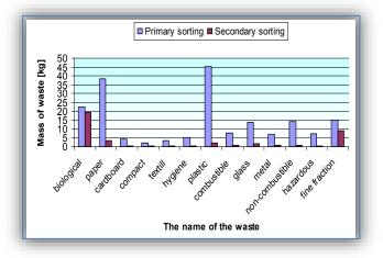
Diagram 4. Composition of remaining waste on the upper and middle sieve examination results
