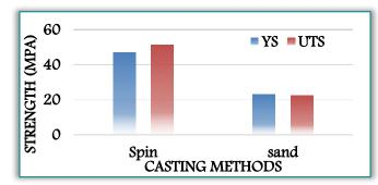
Figure 1. Tensile strength of cast AA6063/SiC, 10% cold~ roll with solution heat-treated
