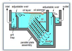
Figure 5. Grease removal [20]
