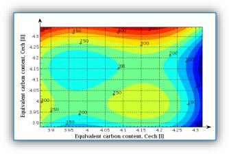
Figure 22. Correlation diagram, case of HB=f(C<sub>ech(I)</sub>,C<sub>ech(II)</sub>)
