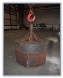
Figure 2: 4000 kg pendulum
