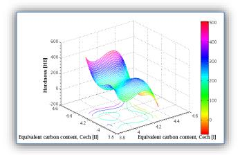
Figure 21. The regression surface, case of  $HB=f(C_{ech(II)}, C_{ech(III)})$
