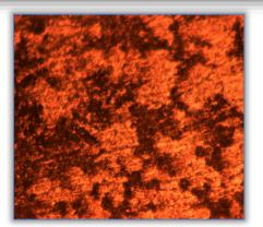
Plate (b) Micrograph of cold rolled and solution heat treated AA6063/SiC for sand casting (X200)
