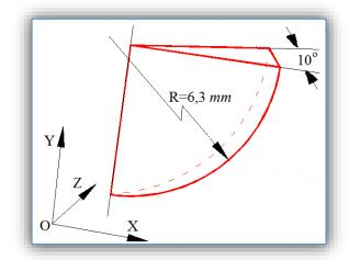
Figure 3: Geometry of the hemisphere sector created to model the 12.6mm rubber ball.
