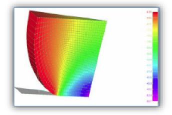
Figure 6:  $\sigma_v$  stress distribution corresponding to an imposed normal approach of 1,42 mm, for the contact between a rubber ball with D = 12,6 mm and a rigid halfspace.
