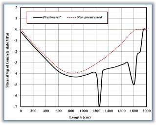
Figure 18. Variation of Stress at top of concrete slab with span length
