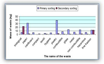
Diagram 1. Composition of remaining waste on the upper and middle sieve examination results
