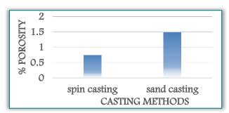
Figure 3: Percentage Porosity for cast AA6063/SiC, 10% cold rolled and solution heat treated
