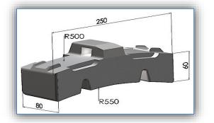
Figure 3. Gray cast iron brake shoes for passenger trains
