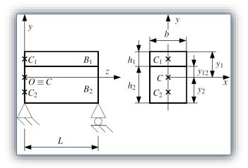
Figure 1. Simply supported bimetallic beam
