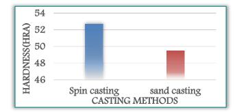
Figure 2. Hardness of cast AA6063/SiC, 10% cold-rolled and solution heat-treated
