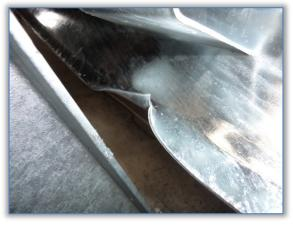
Figure 10: Slide broken in the area of pillar
