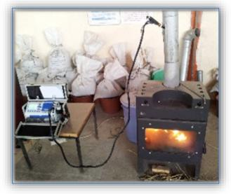
Figure 3 ~ Gas emission measurement test
