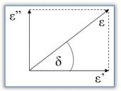
Figure 1. Loss tangent vector diagram Drawing complex permittivity in a simple vector diagram (Figure 1) the real and imaginary part are 90° out of phase.
