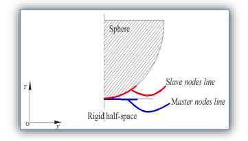
Figure 5. Nodes corresponding to the master and slave sliding lines.
