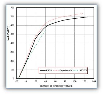
Figure 15. Load-increase in strand force for beam, B2 **Discussion of results for beam B1**
