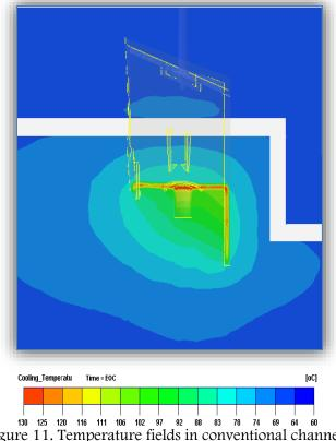
Figure 11. Temperature fields in conventional channels cooled mould after 20 sec. of cooling time (longitudinal cross-section)
