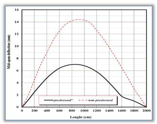
Figure 17. Variation of Mid-span deflection with span length
