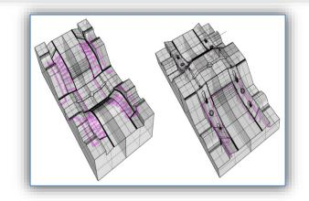
Figure 15. Final design of the injection mould with conformal cooling (A and B blocks)
