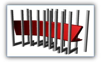
Figure 6. Design of the conventional cooling channels
