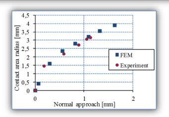
Figure 13: Comparison between the contact area radii obtained experimentally and FEM simulations, for the contact model between a D = 12,6 mm rubber ball and a rigid half-space.
