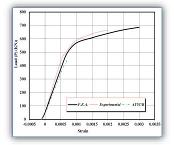
Figure 10. Load-strain curve at top of the concrete slab surface for beam, B1
