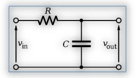
Figure 1. RC Low pass filter The capacitor reactance of an ac circuit is given by:
