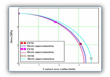
Figure 8: Interpolation of the FEA results for comparison to Hertz contact model.
