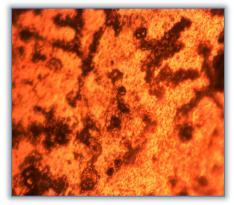
Plate (c) Micrograph of as-cast spin casting for AA6063/SiC (X200)
