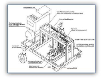
Figure 4 – Arrangement of mechatronic dibbling machine concept
