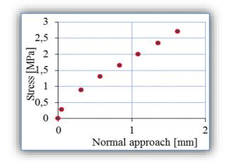
Figure 11. Correlation between maximum stress value and normal approach for the contact model between a  $D = 12.6 \text{ mm} \sim \text{rubber ball and a rigid half-space.}$
