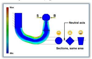
Figure 7: Different sections for towbar
