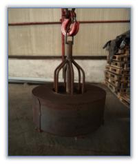
Figure 1:2780 kg pendulum
