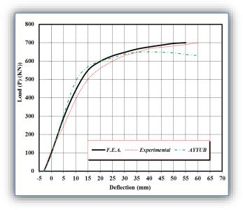
Figure 9. Load deflection results for beam, B2
