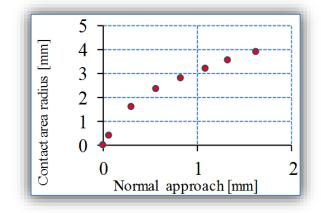
Figure 10: Correlation between contact area radius and normal approach for the contact model between a  $D = 12.6 \text{ mm} \sim \text{rubber ball and a rigid half-space.}$
