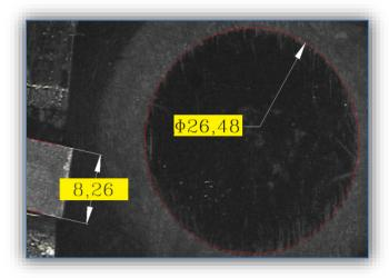
Figure 12: Contact area for an applied load of 13.05N, corresponding to a normal approach of 0.64mm
