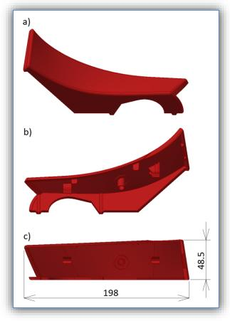
Figure 4. CAD model of the cover from: a) front side, b) back side, c) dimensioned view Cover is made from ABS Novodur P2H-AT with wall thickness in range of the 1 - 3 mm. Injection shot volume is around 44580 mm<sup>3</sup> and part weight is 0,03 kg.
