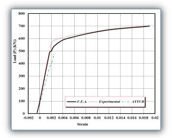
Figure 12. Load-strain curve at bottom fiber of steel beam, B1
