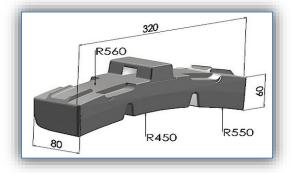
Figure 4. Gray cast iron brake shoes for freight wagons
