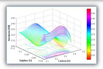
Figure 13. The regression surface, case of HB=f(C,S)
