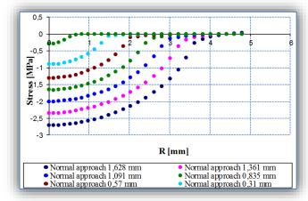
Figure 7:  $\sigma_v$  stress distribution along radial direction, corresponding to several imposed normal approach values, for the contact model between a  $D = 12,6 mm \sim$ rubber ball and a rigid half-space.
