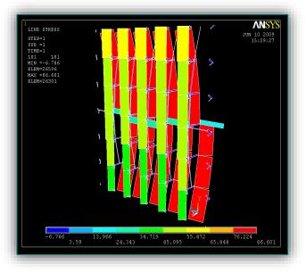
Figure 13. Stress in support structure
