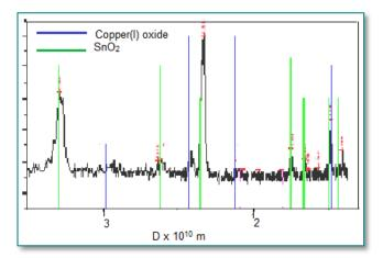
Figure 2. XRD spectrum of the 200 nm thin Cu<sub>2</sub>O film. **Table 1.** Cu<sub>2</sub>O peak identification and D • 10 00 000000
