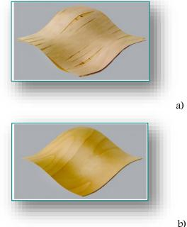
Figure 1. Three-dimensional (3D) veneer plywood produced by bending, from: a) peeled veneer b) mechanically modified veneer [5]
