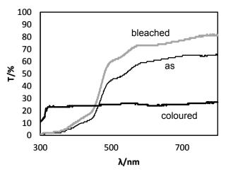
Figure 3. Transmittance spectra of the Cu<sub>2</sub>O film. prepared film, film in colored and film in bleached state taken in-situ: spectra were taken within the The films prepared by the electrodeposition method ECTD and then subtracted with a blank probe. A change in transmittance of film in bleached and colored state is around 53%:
