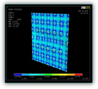
Figure 21. Stress distri. in panels\*(hig. temp)
