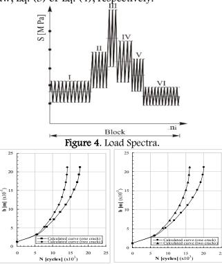
Figure 5. Crack length versus number of loading blocks. The comparison presented in Figure 5 implies that developed computational model based on the crack growth law expressed by Eq.(1) gives slightly lower number of loading blocks up to failure than the one where Eq.(2) is employed.
