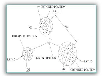
**Figure 4**. Measurement of the positional accuracy of multidirectional motion
