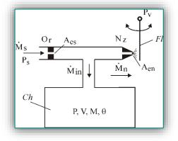
Figure 1. Pneumatic flapper-nozzle with the load chamber
