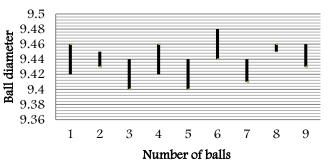
Figure 2. Changes in size balls after dismantling the bearing
