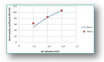
Figure 4. Comparison of the numerical model and experimental results for the heat transfer coefficient for the downwind side of the perforated plate
