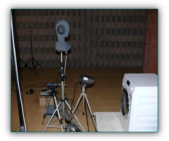
Figure 3. Binaural measurement of washing machine sound
