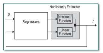
Figure 1. Structure of Nonlinear ARX Models.
