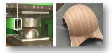
Figure 3. The process of making 3D plywood with male and female template[8]
