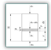
Figure 1: Stresses applied to a powder slice EXPERIMENTAL STATION
