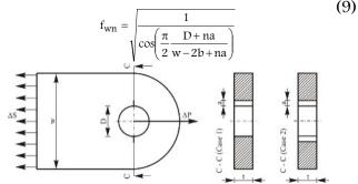
Figure 1. Geometry of the lug with through-thethickness crack.
