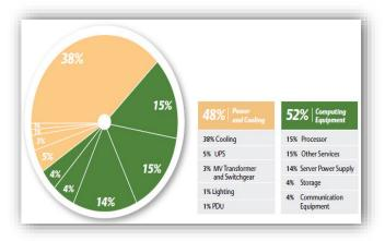
Figure 1. Data-com equipment accounts for over 50% of the energy used while power and cooling account for an additional 48% in a traditional data centre
