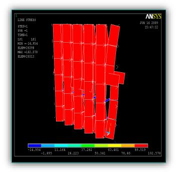
Figure 17. Pre-tension 100MPa\*(nom.temp)
