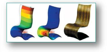
Figure 7. The software analyzes the load of the seat and backrest with chairs "XUS" (Designer: Peter Karpf, a Dane, Producer: iform, plugs) [7]
