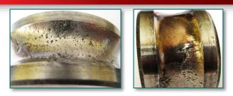
Figure 3. Fatigue wear (pitting) on the outer surface of the bearing inner track
