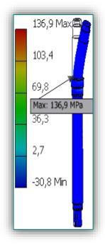
Figure 4. Distribution of the 1-st principle stresses
