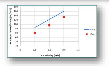
Figure 3. Comparison of the numerical model and experimental results for the heat transfer coefficient for the upwind side of the perforated plate
