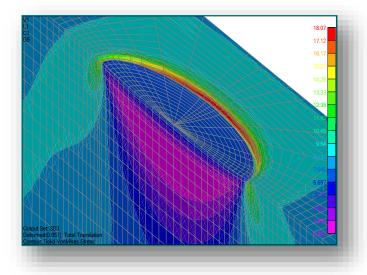
Figure 2. Detail finite element model of semi-elliptic crack
