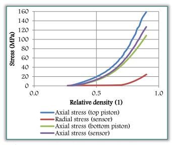
Figure 4: Evolution of the axial and radial stresses during compaction
