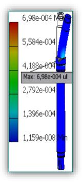
Figure 5. Distribution of equivalent strain
