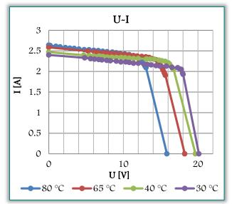
Figure 4. U-I characteristics in different temperatures
