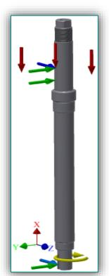
Figure 2. Loading of the spindle The following characteristics of the finite elements mesh were set: average element size 0.1; minimum element size 0.2; grading factor 1.5; maximum turn
