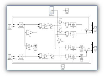
**Figure 2**. Block diagram of the control system of level and temperature in decoupled flow tank with introduced disturbance
