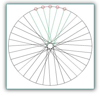
Figure 9. Seven altered spokes without additional examined points
