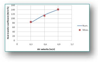
Figure 5. Comparison of the numerical model and experimental results for the overall heat transfer coefficient
