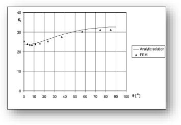
Figure 3. Comparisons between analytic and FE results for SIF calculations
