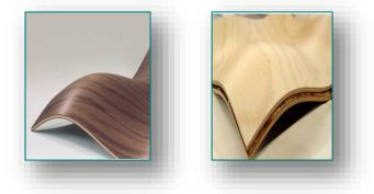
Figure 2. Trodimenzionalne (3D) furnirske ploče [7] peeled veneer beech, or sliced veneer beech, all kinds of walnut, oak or cherry, which were previously mechanically modified, so they texture remains unchanged. The inner layers are made of peeled beech veneer. The thickness of threedimensional plywood range from 1.5 to 20mm. Veneers are glued to plywood (molding) in a mold (template) with male and female or in diaphragm presses by applying the UF glue for hot or cold bonding. [7]
