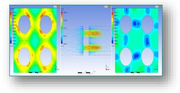
Figure 7. Numerical results for the Reynolds number 300 - air velocity of 1,24 m/s
