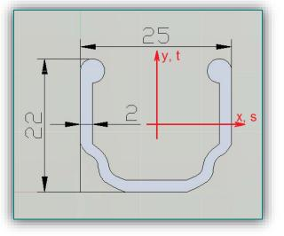
Figure 1. Cross section of the rim The Saint-Venant torsional constant I<sub>T</sub> is calculated by the formula valid for thin-walled open cross section [6]:
