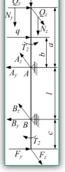
Figure 1. Scheme of loading of the cutting spindle Static analysis
