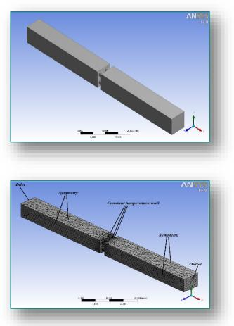
Figure 1. A 3D model and its numerical grid with boundary conditions
