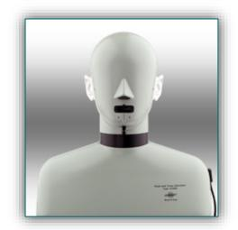
Figure 2. Binaural measurement system – artificial head (Head acoustics and Brüel & Kjær) [4, 5]
