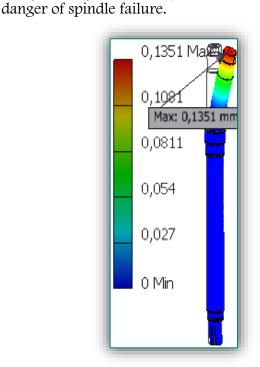
Figure 7. Distribution of resultant displacement
