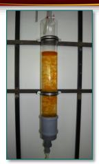
Figure 4. The reaction column for coagulation
