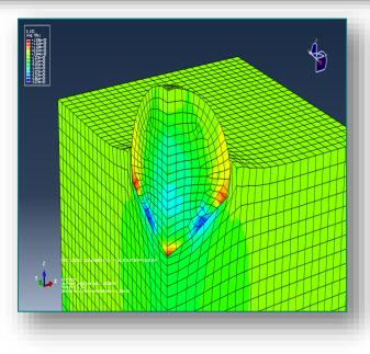
Figure 2: Peening stress at 1540 [K] at an impact speed of 450 [m / s]
