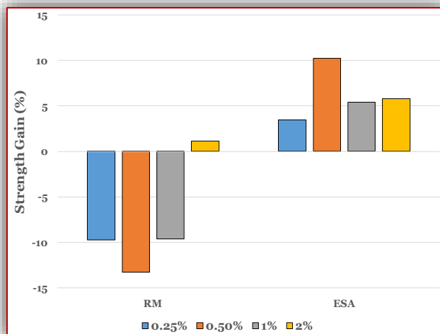
Figure 6. Percentage Early Strength Gain of ICL Stabilized Soil admixed with RM and ESA
