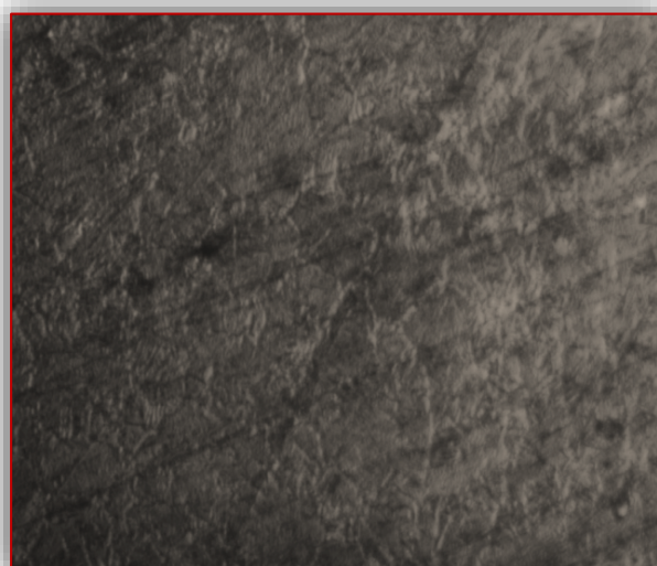
Plate 3: Microstructure of sample C 40 percent by volume of PEG (after quenching operation) – 200X
