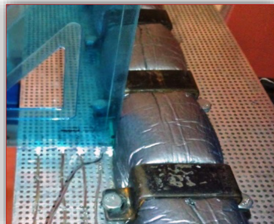
Figure 4. Thermocouples positions on the perforated plate
