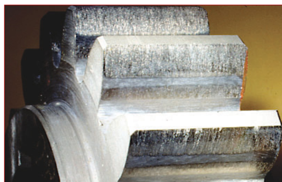
Figure 7. Gear scuffing failures [12]
