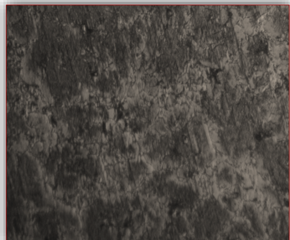
Plate 2: Microstructure of sample B 60 percent by volume of PEG (after quenching operation) – 200X
