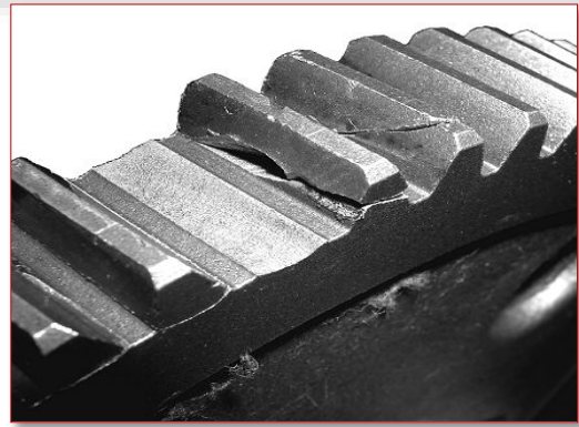
Figure 10. Breakage of more gearteeth [15]
