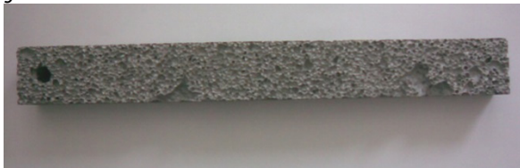
Figure 3. The metallic foam beam
