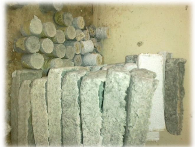
Figure 2: Flexural and compressive samples of cement bonded white and brown paper boards
