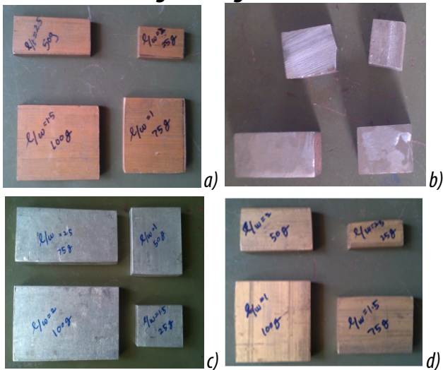
Figure 2. Parts of different material with different L/W Ratio and mass: a) copper; b) steel; c) aluminum; d) brass
