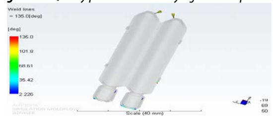
Figure 13. Weld line defect
