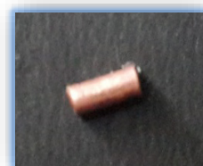
Figure 5. Aluminium and Copper billets (38 μm grain size)
