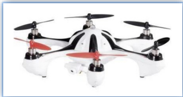
Figure 1. Hexa-rotor microcopter used for the experiments The autonomous hexa-rotor microcopter, Figure 1, consists of six rotors attached to a rigid body frame and these additional two rotors make it able to carry:
