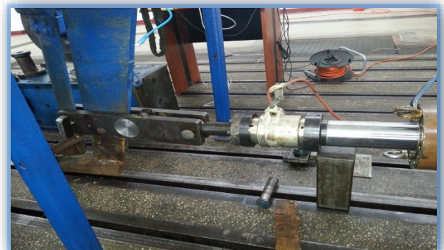
Figure 6. Testing stand of deep soil loosening machine MAS 65, coupling detail of force cylinder to machine working part
