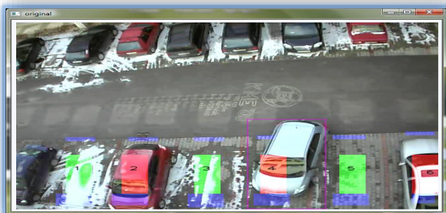
Figure 5. Detected movement of persons does not affect the change of parking space occupancy (left), a vehicle detected release a parking space (right)
