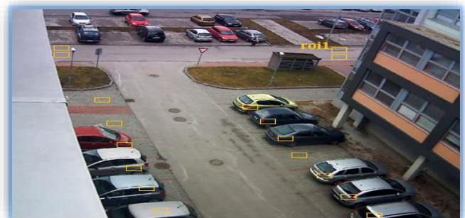
Figure 4. Proposed deployment of ROIs among sectors (left); an example of ROIs deployment in the monitored sector, aimed at motion detection (right) DIFFERENT OCCUPANCY STATUS OF PARKING SPACES
