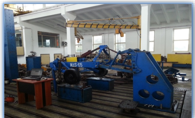
Figure 5. Testing stand of deep soil loosening machine MAS 65, general view
