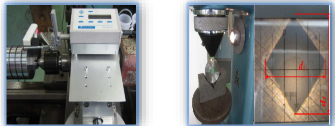
Figure 4. Measurement of roughness with a profilometer and the Vickers hardness measurements
