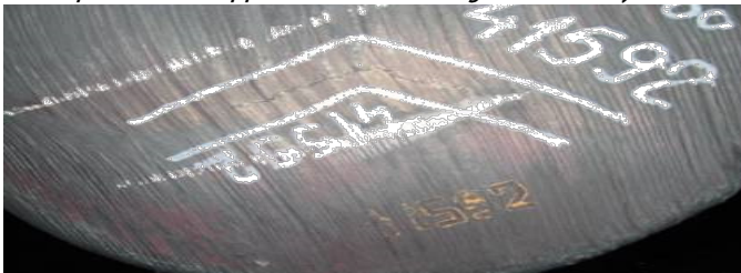
Figure 7. Internal fissures in the centre
