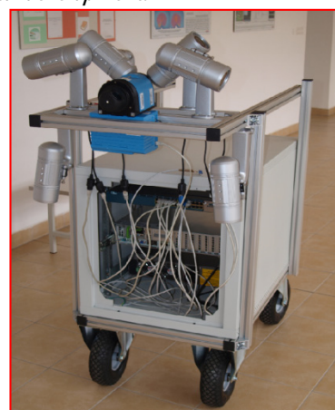
Figure 1. Mobile measurement platform (MMP)
