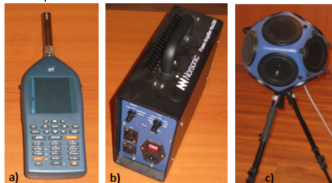
Figure 4 a) Sound level meter NORSONIC Nor 140. b) Noise generator Nor 280, c) Omnidirectional sound source NORSONIC 270
