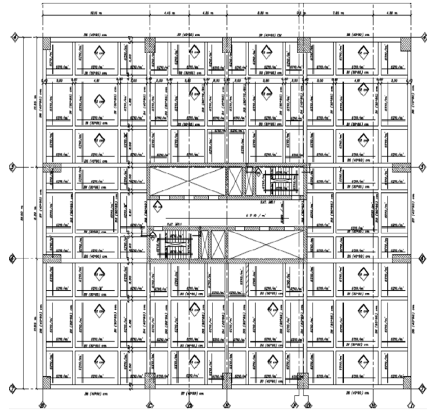
Fig. 4 Paneled beams slab plan system
