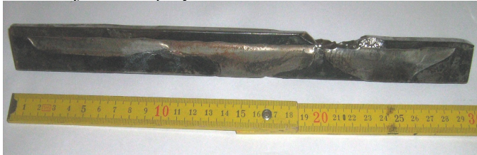
Figure 2. Damaged extraction cage knife - made by cladding
