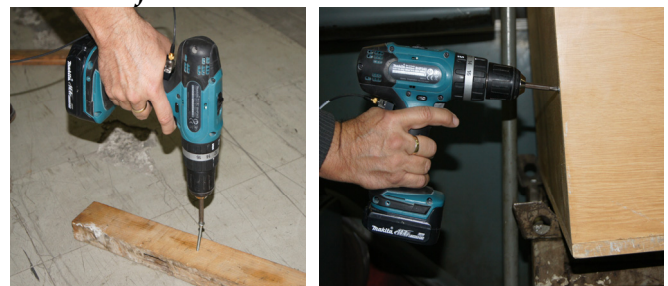
Figure 10. Machine C- Cordless Drill Driver ( \Phi 5 ) Working with Cordless Drill Driver in vertical and horizontal positions
