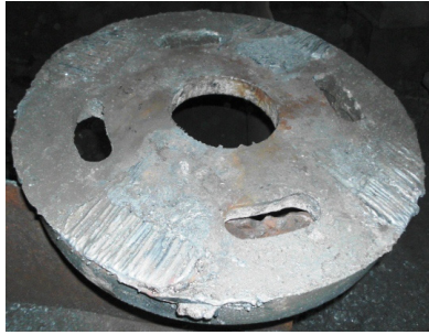
Figure 17. External surface of the real casting without shrinkage porosities
