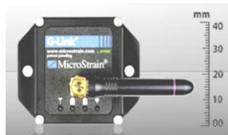
Figure 3. Wireless Accelerometer Node
