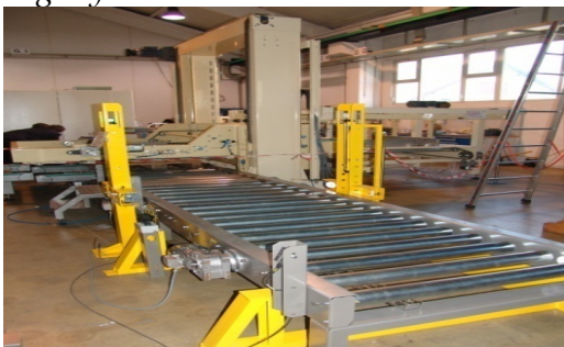
Figure 3. Transport rollers for transporting piles with sensors [8]
