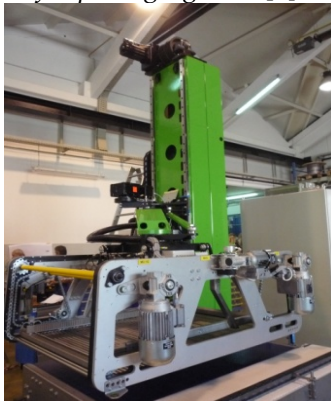
Figure 2. Paletizer for for piling packages [8]
