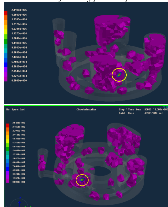
Figure 15. The phenomenon of the Hot Spot can be seen in the simulation by the Modulus method and the Heuver's method.
