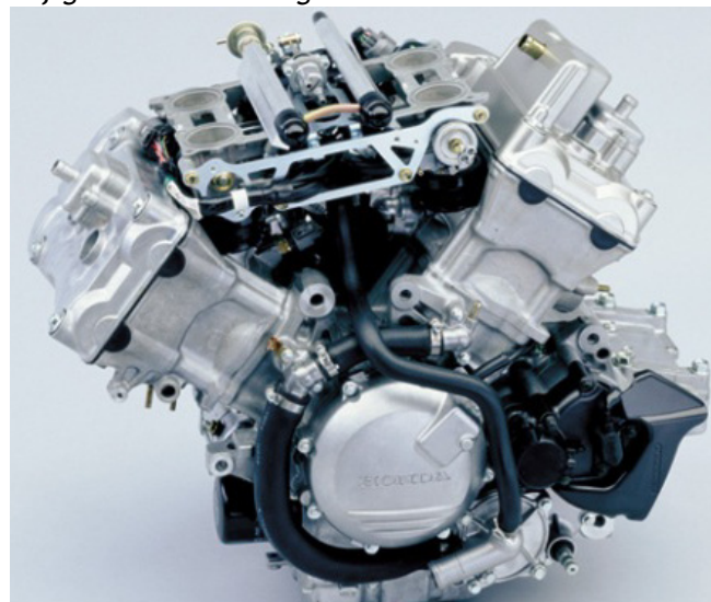
Figure 1. The engine of the tested motorcycle Honda VFR 800 - left side [17]
