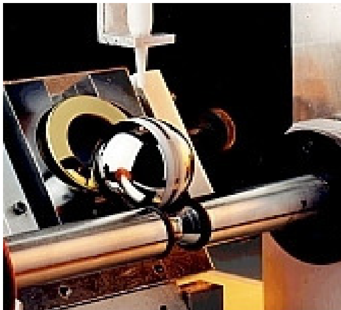
Figure 4. Rambling ball tribometer [6]
