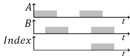
Figure 1. The typical signals of the incremental encoder
