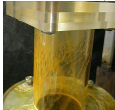
Figure 15. Fuel jet diffusion into the cylinder at high lift and speed
