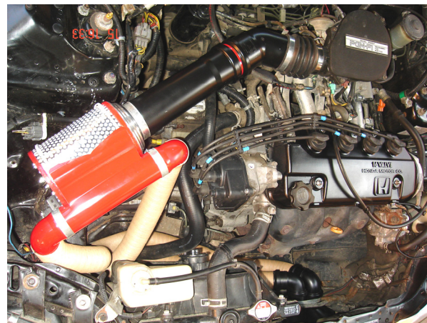
Figure 10. DATD, bi-route mounted on Honda Civic, 1.6
