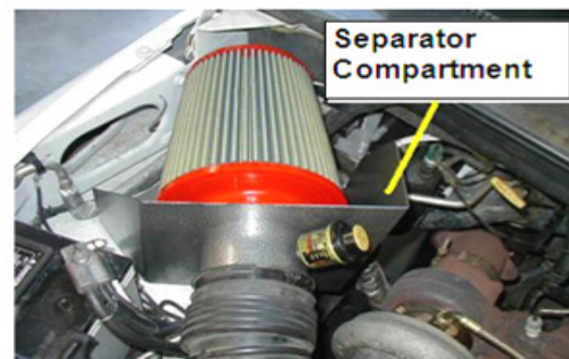
Figure 1. Assemblies that lead to direct exposure of the filters
