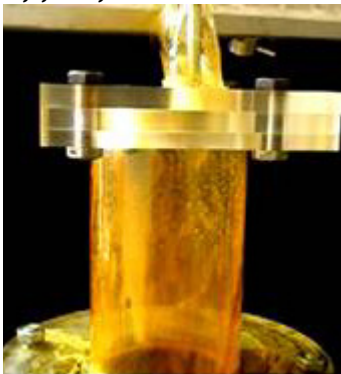
Figure 9. Fuel film diffusion into the cylinder at the back valve in spray mode
