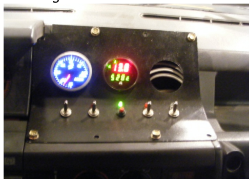
Figure 1. Commands board for programmable ECU, inside the vehicle
