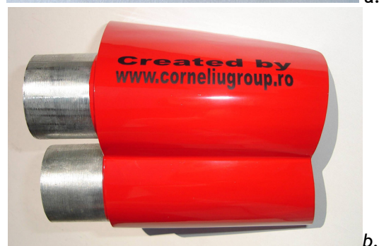
Figure 6. Axial external collector a - mono-route, b - bi-route
