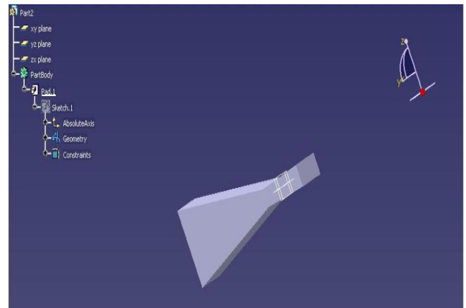
Figure 3: Geometry of rectangular straight nozzle
