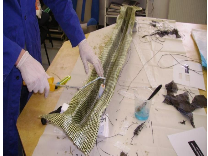
Figure6: Kevlar-carbon fibre laying in the mould Prepared and saturated fibres have been placed into vacuum and they got hardened (Figure 7). After the material hardened, the work layers were getting off. The surface of one side was adjusted for deformation elements connection and the other side for better look.
