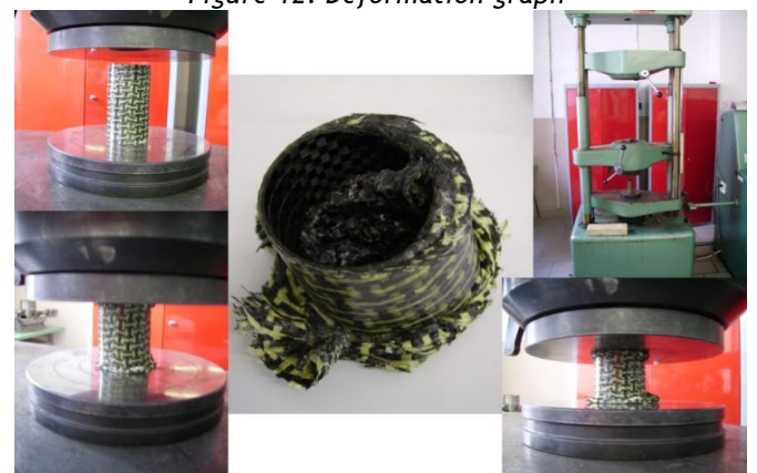
Figure 13: Deformation element testing
