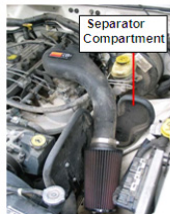
Figure 2. Installing filters in separator compartments
