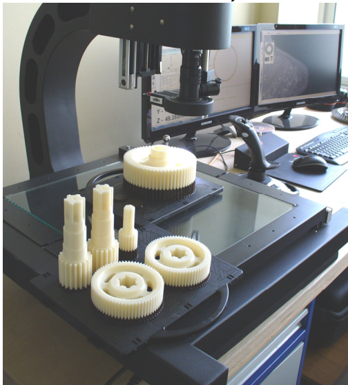
Figure 3. The coordinate measuring system - BATY VENTURE
