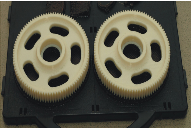
Figure 6. FDM models of gears the planetary gear's
