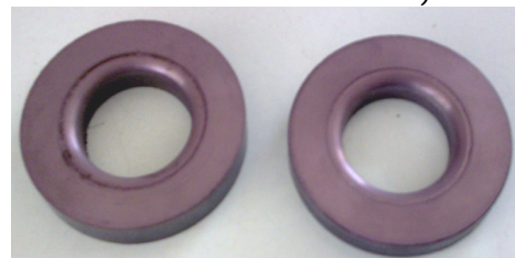
Fig.9 - Blank holder (a) and die (b) manufactured by composite material 96%Fe and 4% Al 2 O 3 compressed by pressure of 600MPa and sintered on temperature of 1150°C
