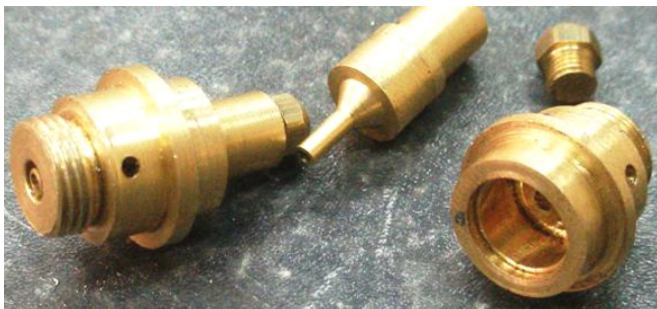
Figure 5: Assembled and disassembled of a Manufactured Injector
