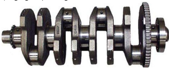
Figure 1. Single-throw crank-shaft of Volkswagen engine 1,8T material EN-GJS-600-3 ( www.lam.mw.tum.de )
