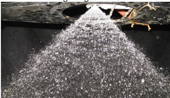
Figure 10: Fully Opened Spray Cone Under design conditions ( P_f=10 , P_o=4 bar)
