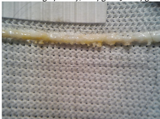
Figure 5 - Laser welded sample, line energy 4.8 kJ/m
