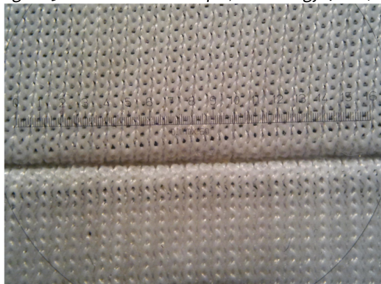
Figure 6 - back side of a laser welded fabric, line energy 4.8 kJ/m
