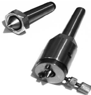
Figure 5 – Standard centre and new solution with fastening screw and setting pins
