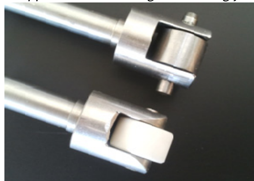
Figure 2 - Different drawing rolls to ensure a well defined thermal contact between textiles. Steel (upper drawing) roll and ceramic roll
