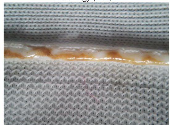
Figure 8 - Laser welded sample with carbonation weld seam, line energy 4.1 kJ/m
