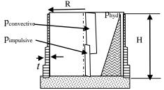
Figure 13. FEM model dimensions
