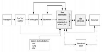
Fig. 2. Mass Customization Configurator for apparel industry
