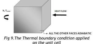
The boundary condition imposed on the unit cell is shown in the Fig.9.
