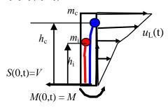
Figure 6. Base shear and overturning moment load on a vessel by seismic action
