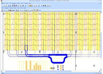
Figure 5 - 2D representation of material flow with Sankey diagram
