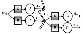
Figure 3 - Diagram of fast wavelet transformation m=3 levels
