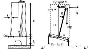
Figure 2. Shell skirt modelling. a) Sketch. b) A 2D two spring one lumped mass dynamical model.
