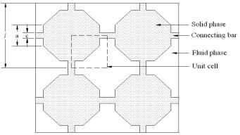
Fig. 5. Two-dimensional spatially periodic two-phase system (Touching octagon cylinder) Because of the symmetry of the plates, one fourth of the octagon cross-section has been considered as a unit cell and is shown in Fig.6.
