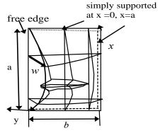
Figure 12. Plate buckling model
