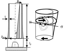
Figure 10. Shell geometry and buckling
