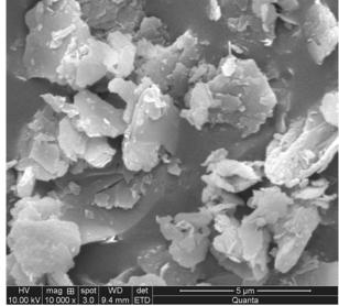
Fig 8 SEM Photo of Kaolinite processed under 500°C for six hours The creation of thermal in some part of structure after construction due to positive affect on the subsoil and
