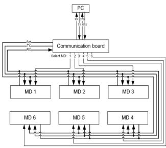
Figure 8 - Communication interfaces in control system
