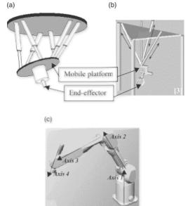
Figure 1 - Examples of (a) fully parallel, (b) hybrid parallel and (c) serial (anthropomorphic) mechanisms
