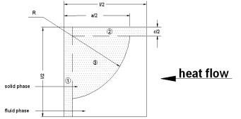
Fig.8. Unit cell of circular cylinder
