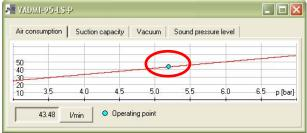
Figure 8 - Compressed air consumption at pressure level 5,2 bar
