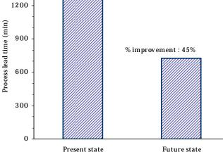
Present state Future stat Figure 11. Reduction of process lead time
