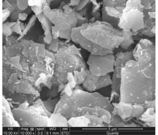
Fig 5 SEM Photo of Kaolinite processed under 200°C for six hours
