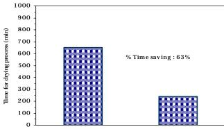
Present state drying process New improved oven drying
