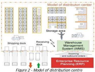
The WMS provides a set of the computerized procedures for handling the receipt of the stock and the returns into the warehouse facility, modelling and managing the logical representation of the physical storage facilities (racks and shelves), managing the stock within the facility and for enabling a link to order's processing in order to pick, packing and shipping goods from the facility according to the customers' demands and organizing deliveries of goods to customers.
