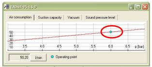
Figure 6 - Compressed air consumption at pressure level 6 bar
