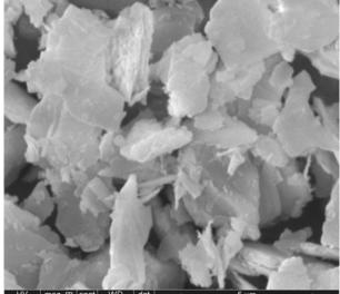
HV mag ⊞ spot WD det \_\_\_\_\_5 µm \_\_\_\_\_ 10.00 kV 10.000x 13.0 22.1 mm ETD \_\_\_\_\_Quanta Fig 6 SEM Photo of Kaolinite processed under 300°C for six hours
