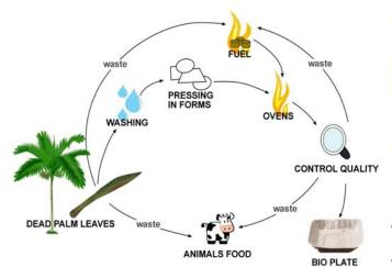
Figure 4 - Simplified systemic BioPlate production process
