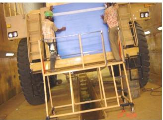
Figure 9. Masking with safety trolley – operator risk eliminated
