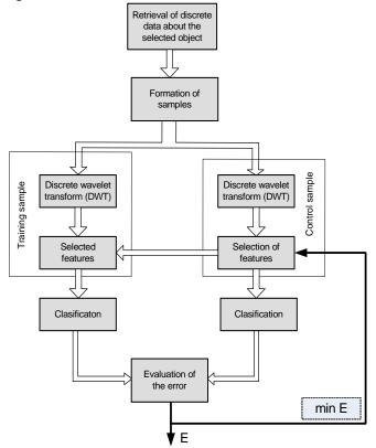
Figure 1 - General structure of the process "synthesis of a classificatory for recognition of metals" with an application of wavelets methods
