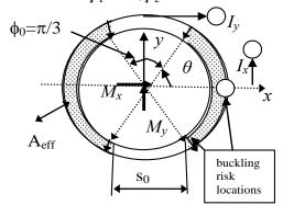
Figure 9. Skirt cross section at opening Decision variable  $s_7 = N_{skirt.cylinder}$  or skirt cylinder buckling safety factor The buckling strength reduction factor
