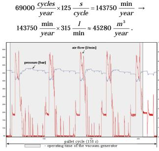
Figure 10 - Consumption of compressed air on the pallet machine in the one cycle
