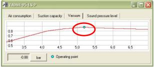
Figure 9 - Vacuum level at pressure level 5,2 bar
