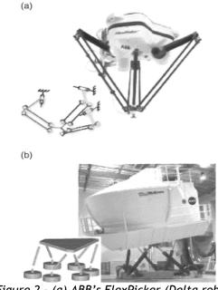
Figure 2 - (a) ABB's FlexPicker (Delta robot); (b) NASA's flight simulator (Hexapod)
