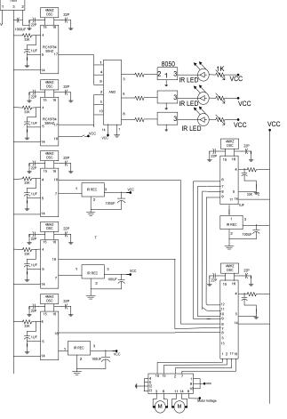
Figure 3: Circuit diagram of the designed controller
