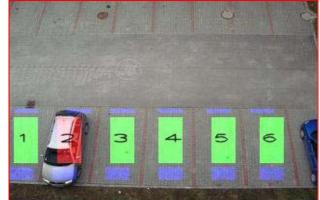
Figure 2. Example of ROI placement for parking places Detection of moving object
