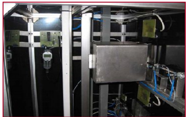
Figure 9: The placement of the SMS card with the attached mobile phone in the model of the elevator.
