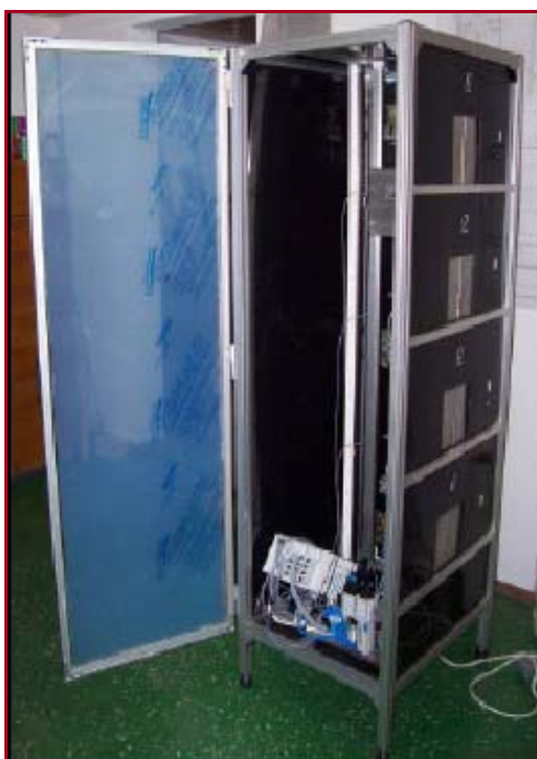
Figure 10: The placement of the SMS card with the attached mobile phone in the model of the elevator
