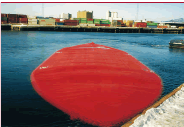
FIGURE 3. Floating tank for collected oils [13]
