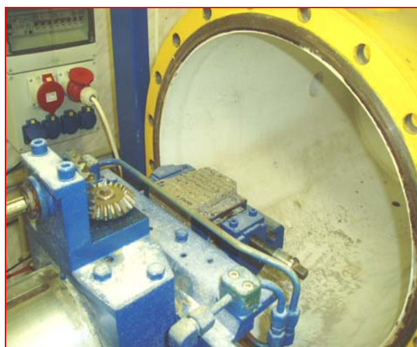
Fig. 1. Support with sample in front of the pressure vessel
