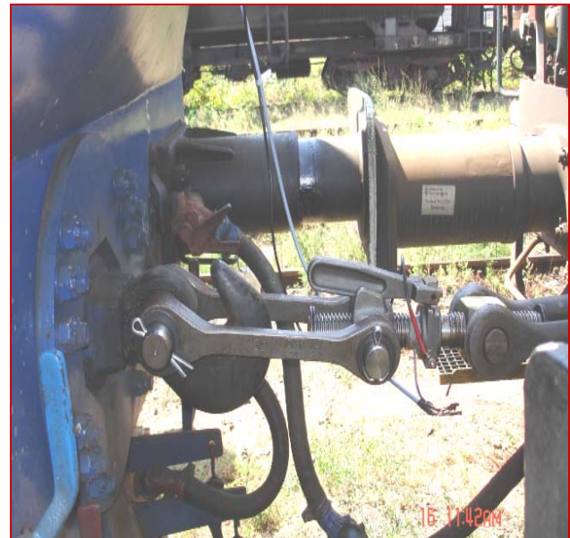
Figure 2 Drawing hook with strain gauges
