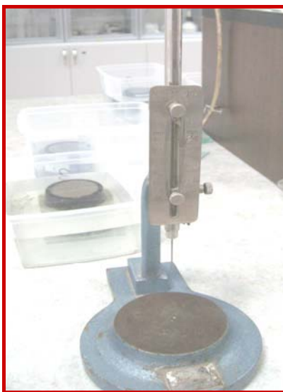
Figure 9. Vicat apparatus for determination of water for the normal consistence paste
