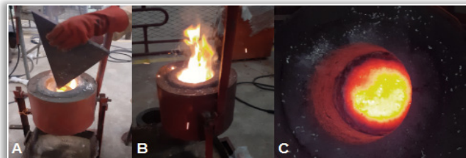
Figure 3. Obtaining of the Termites: A) Reactor feed and ignition of the reaction, B) Self-sustainability of the reaction, C) Cooling of the termite
