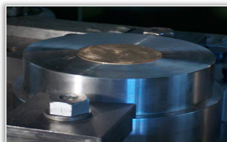
Figure 18. A view of the Blank on the Lower Supporting Die
