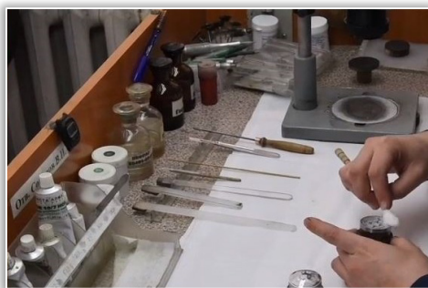
Figure 8. Manual polishing of coin dies
