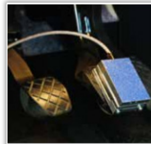
Figure 5. Brake pedal force measurement sensor [12]
