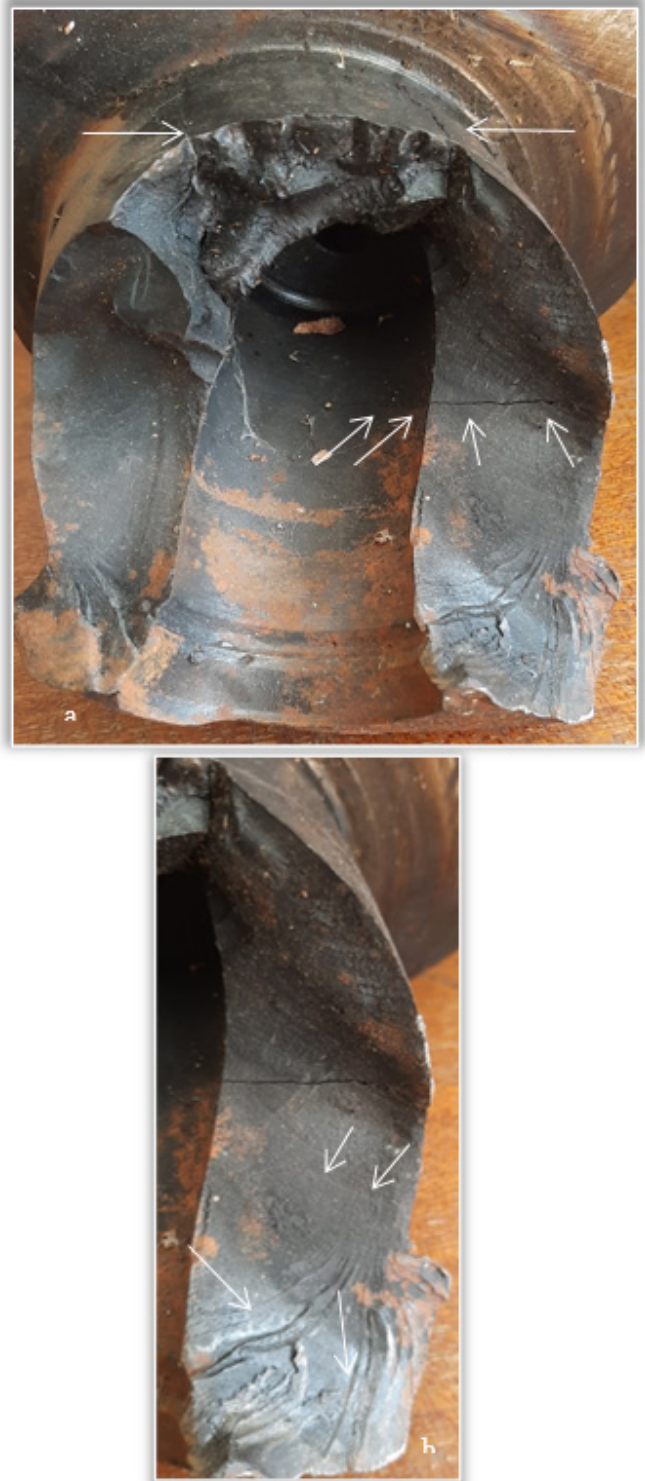
Figure 4. Destroyed cast iron crankshaft from a truck: a) secondary cracks "open type" b) Rivers marks.
