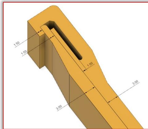
Figure 4. Wall thickness
