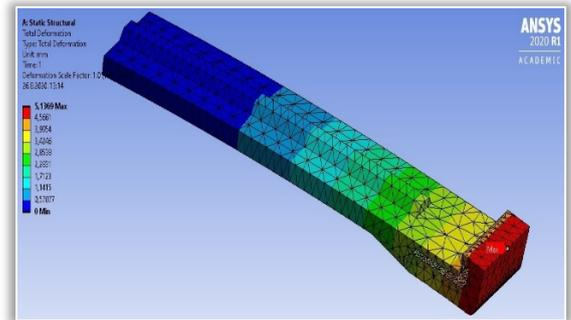
Figure 11. The total deformation on the inside of the buckle
