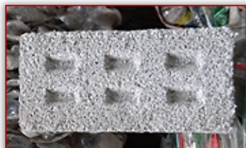
Figure 5. A recycled plastic brick
