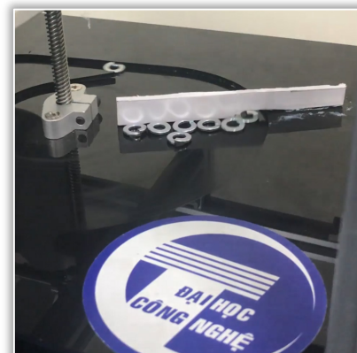
Figure 6. Classification mechanism for washers
