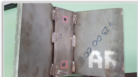
Figure 6. Appearance of the corner-edge joint with protection: a) at the entrance side, b) at the exit side.
